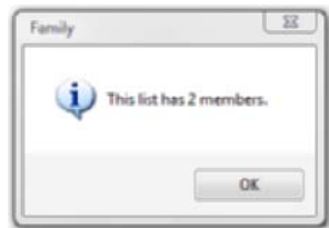
→ Figure 7.13 The MsgBox method displays a message to the user, with optional title and icon.
