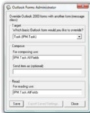
Figure 21.6 Use the free Forms Administrator tool to help modify the registry so that a custom form can replace a standard form as the global default.
