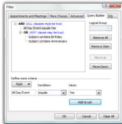
→ Figure 16.2 The Query Builder tab adds the ability to construct complex searches with both AND and OR operators.
