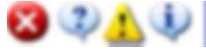
Figure 8.8 From left to right, the Critical Message, Warning Query, Warning Message, and Information Message icons.
