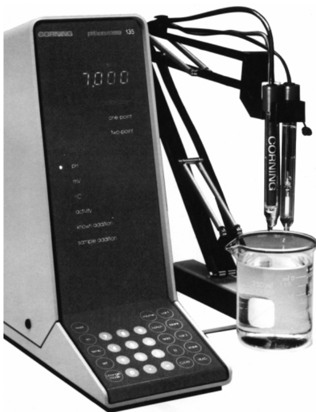
FIGURE 5-8 A modern microprocessor-controlled pH meter.
