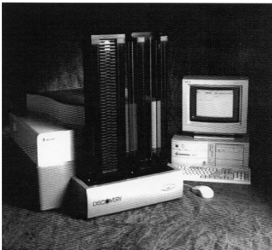
Figure 5 Discovery HTRF Microplate Analyzer. (Courtesy of Packard Instrument Company, Meriden, CT.)
