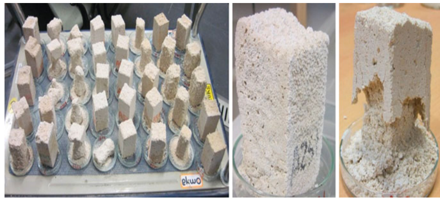
Fig. 7 General view of mortar samples at 42 cycles after chlorides contamination and zoom view of an AL mortar sample only with superficial disaggregation and a PL mortar sample with great mass loss
