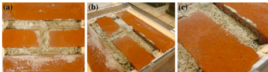
Fig. 2 Surface of MA wallette after 7 weekly cycles: (a) after brushing (b–c) details of MA specimen after 7 weekly cycles: severe scaling of the mortar can be observed
