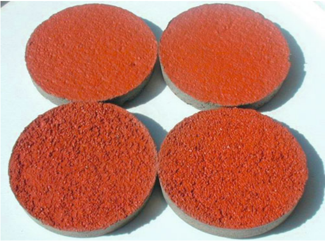
Fig. 15 Samples of the finishing coats used to characterize the optical and radiative properties
