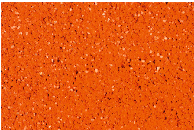
Fig. 34 Observation point P3—Opening of the pores of the finishing coat at ageing time T2.1 (i.e. after UV and winter cycles, but before summer thermal shock cycles during ageing time T2)
