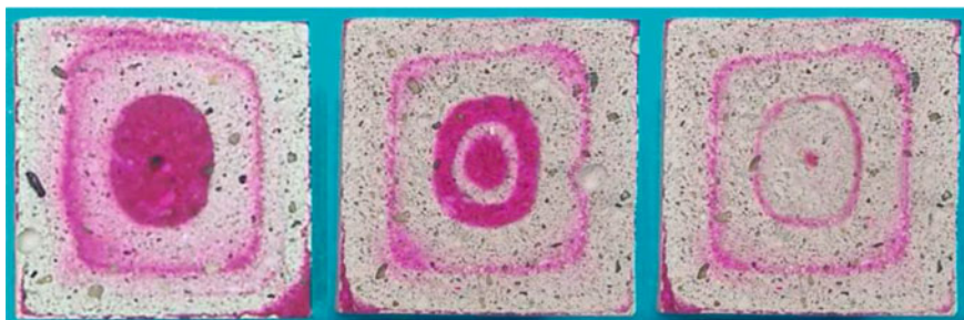
Fig. 4 Fracture surfaces of LG specimens, tested with an alcoholic solution of phenolphthalein: from left , carbonation depth at 7, 14 and 28 days of exposure to accelerated environment
