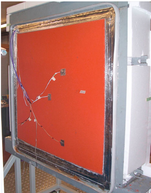
Fig. 30 The big sample (1 m 2 ) applied as door to the weathering chamber before ageing (T0)
