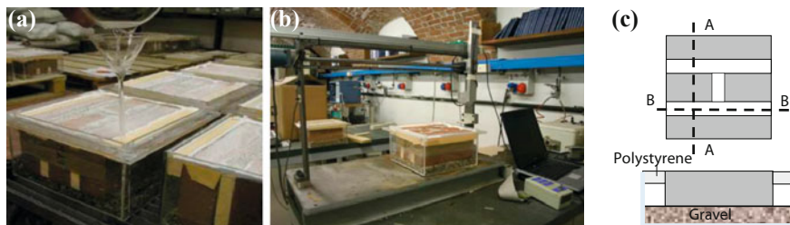
Fig. 3 a wallettes in the boxes, b laser profilometer, c scheme of the measurement
