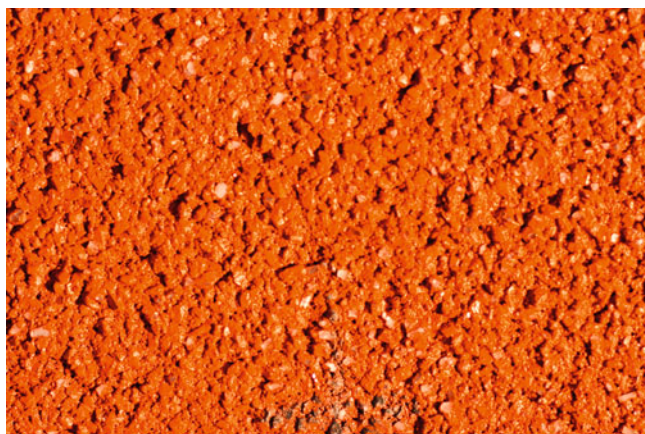
Fig. 33 Observation point P3—Opening of the pores of the finishing coat at ageing time T1.1 (i.e. after UV and winter cycles, but before summer thermal shock cycles)
