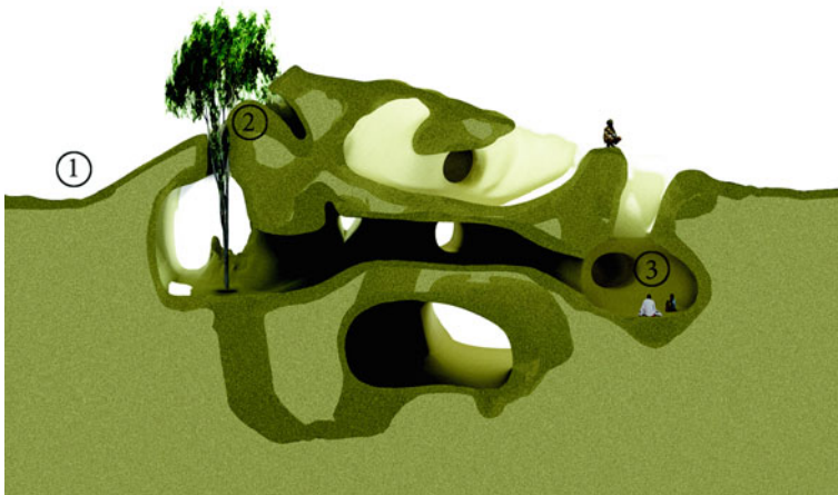
Fig. 8 Performative section: The habitable sandstone structure adds a roughness to the surface texture of the dune (1), provides physical support for the shelterbelt trees (2), and creates habitable spaces inside of this barrier (3)
