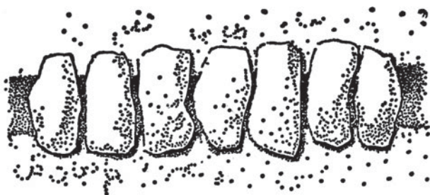
▲ Fig. 114. Capstones cover aqueduct to prevent evaporation.
