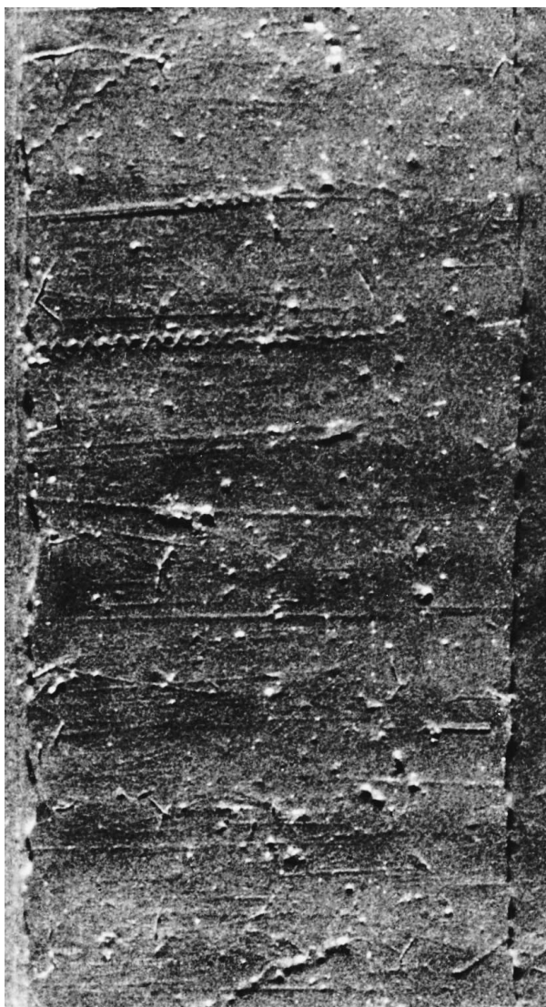
Figure 9 A different section of the cast shown in Fig. 8, further along the heat-sealed plastic bag. The silicon arm, which is pressed down on to the plastic bag during the heat-sealing process, has numerous minute defects whose spatial orientation produces a unique pattern, readily recognizable on any surface (or a cast thereof) that has been sealed by it.
