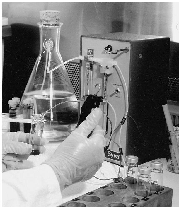
Figure 3 Automatic diluter apparatus for mixing blood samples with ISTD solution.
