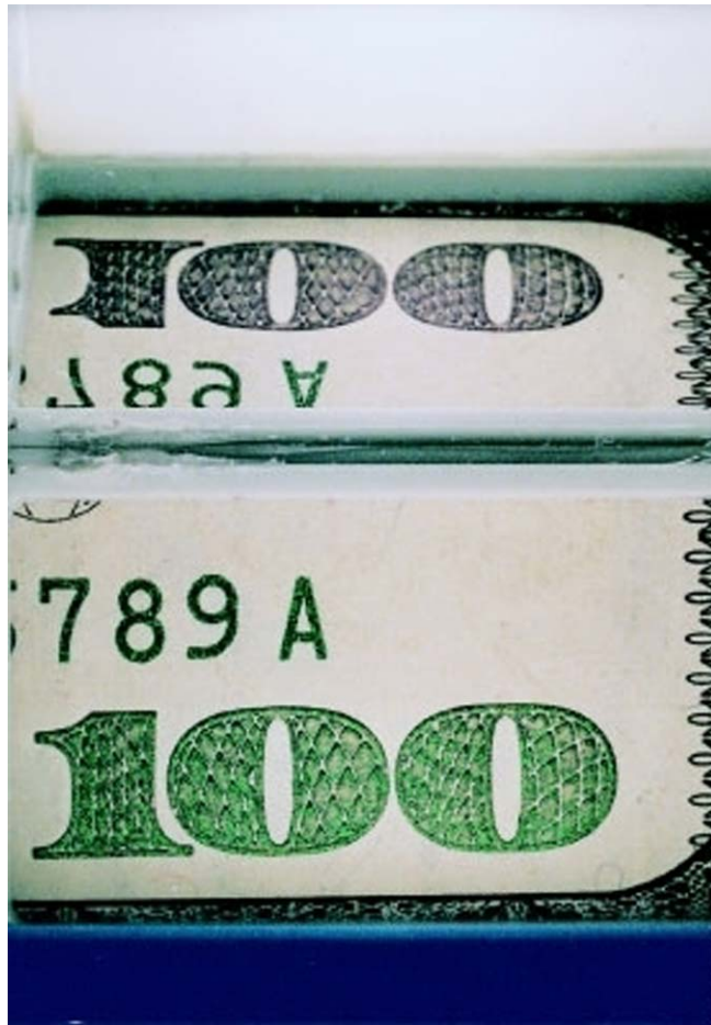
Plate 27 FORGERY AND FRAUD/Counterfeit Currency Green-to-black color shifting link on genuine US banknote. Photographed using an angled mirror: green image (below) at normal; black (above) at an oblique angle.
