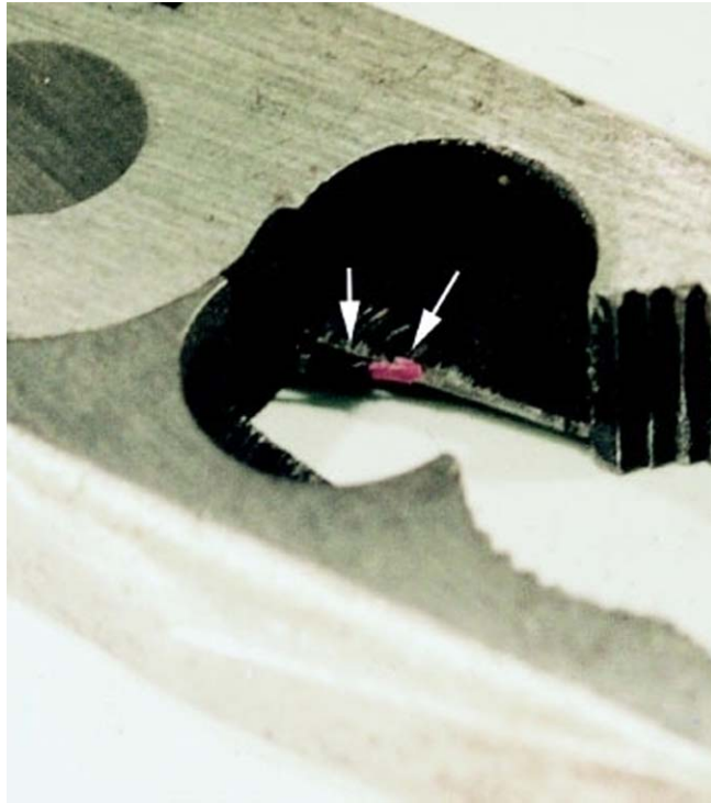
Plate 44 PATTERN EVIDENCE/Tools Macrophotograph showing multicolored plastic insulation material caught in cutter blades of suspect pliers.
