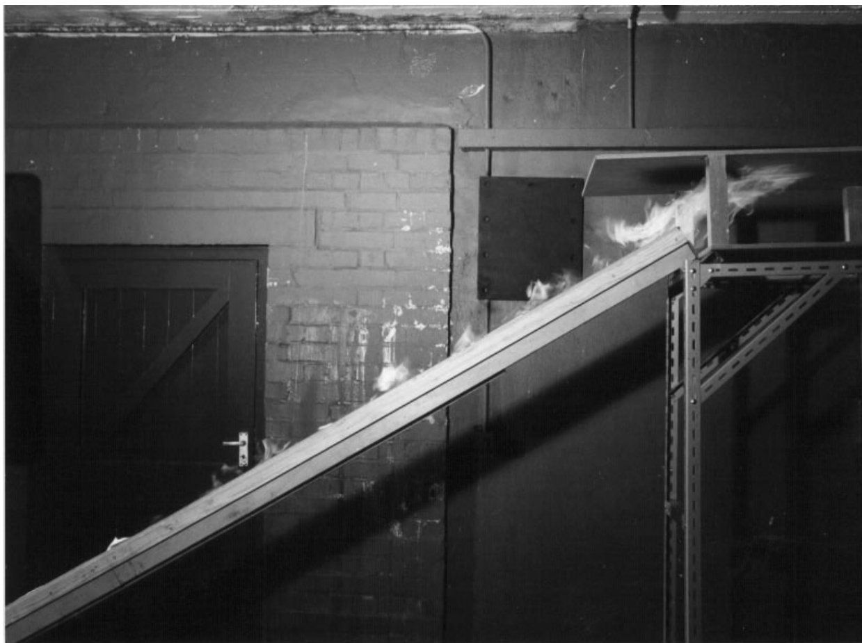
Figure 3 Fire tests on scale models of the escalator troughs at Kings Cross were conducted by the Health and Safety Executive at Buxton to demonstrate how the flames lay low in the trough with a jet of flame at the top – the 'trench effect'. Investigation into the Kings Cross Underground Fire, Desmond Fennell QC Cmm 499 HMSO London (1988). (Crown Copyright.)
