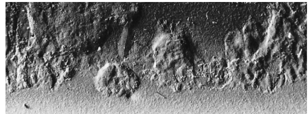
Figure 13 A second cast collected from the scene (Fig. 11) was initially discarded, because of what was perceived to be poor detail. The unusual pattern seen in this second scene cast, however, could be related directly back to a specific section on the second implement, a drop forged crowbar.
