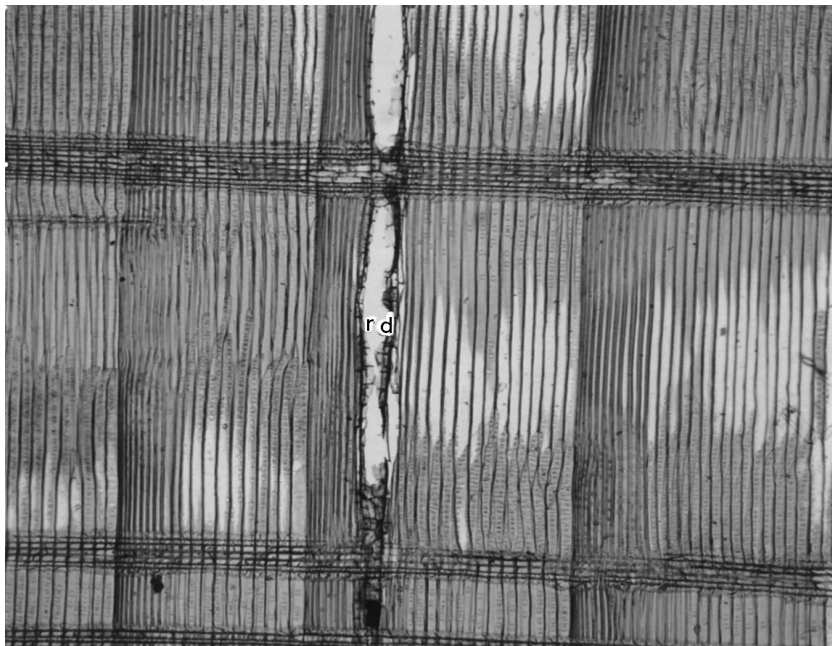
Figure 10 Radial section of softwood Prunus resinosa showing 'brick wall' of rays. rd, resin duct. Resin ducts are essentially empty tunnels, surrounded by a layer of epithelial cells unlike vessels which consist of tubular elements. Original magnification \times 40 .
