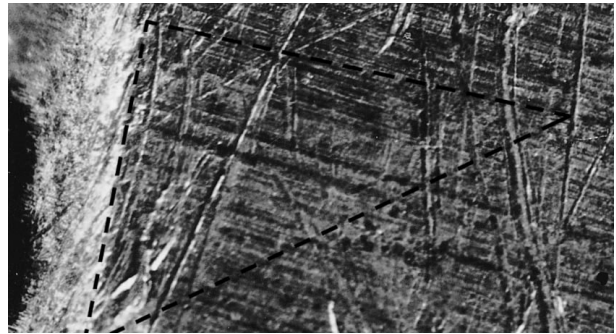
Figure 12 A photograph of a portion of one side of a small screwdriver recovered from one suspect. The detail is located some 12 mm from the actual screwdriver blade and shows both machining and wear features (see Fig. 11).
