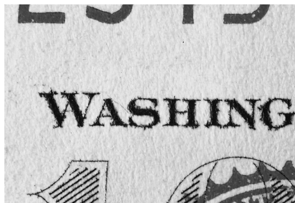
Figure 1 Intaglio printing on genuine US banknote.
