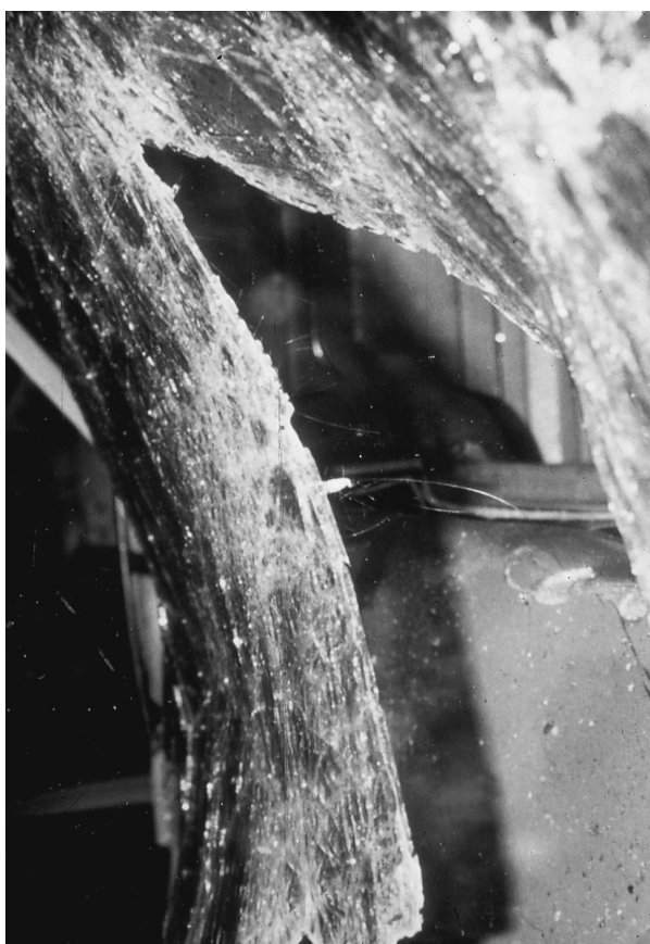
Figure 14 Occupant contact with the front windshield may reveal the transfer of hair, blood and tissue. This evidence can be matched to the standards obtained from the occupants.
