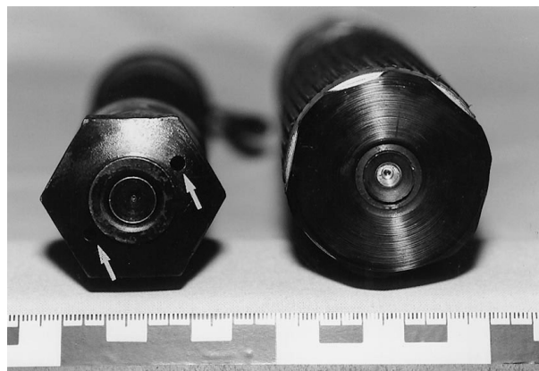
Figure 2 Muzzle end of two captive-bolt stunners. Left: Kerner type with two opposite openings (outlets for the explosion gases; arrows); right: Schermer type without additional smoke conduits.
