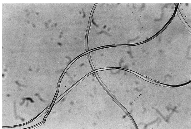
Figure 2 Silk fiber (magnification 90×).
