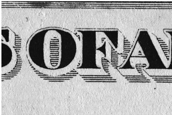
Figure 20 Counterfeit US $100 FRN: printed offset.
