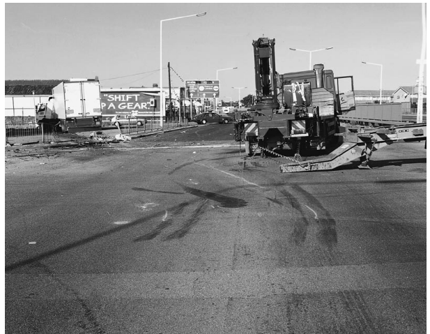
Figure 1 Tire marks scrapes and gouges can be seen in the roadway following this incident involving two goods vehicles. © Metropolitan Police Service.
