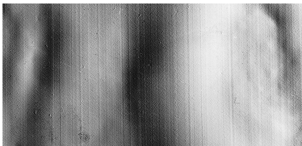
Figure 1 Case study 1. A cast of the inner surface of extruded irrigation piping. Extruded striae are quite common on a wide range of materials, including plastic bags, copper wiring, etc., and may allow a relationship to be demonstrated between two sites (objects). The major concern with such evidence relates to the length over which such comparable striae are left. A study of the manufacturing process and the quality controls in place, as well as samples from the manufacturer, should always form part of any such identification work.
