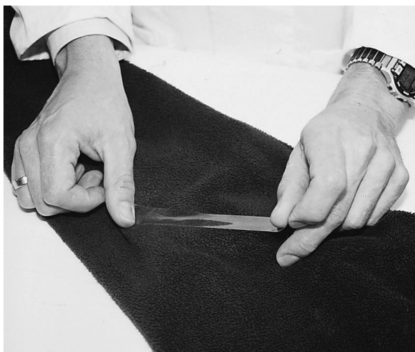
Figure 1 (see color plate 21) Recovering fiber debris from a garment using clear adhesive tape.
