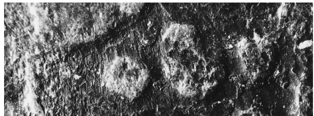
Figure 14 A small section of crowbar identified by a thin smear of aluminum. In this location scaling and other individual features left on the bar during its manufacture were directly comparable, even though a slight dragging of the crowbar across the surface had occurred (see Fig. 13).
