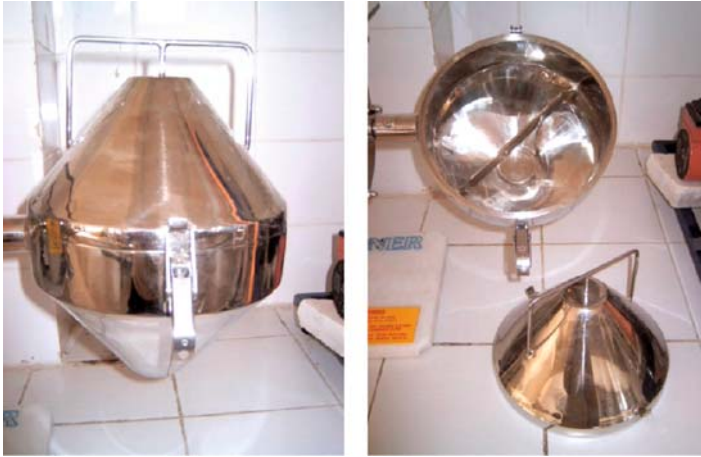
Figure 1.5. Cone type tumbling mixer; on the left, cone view; on the right, inside view of cone.
