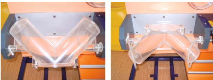
Figure 1.6. V-shape tumbling mixer on the left, mixer up view, on the right, mixer down view.
