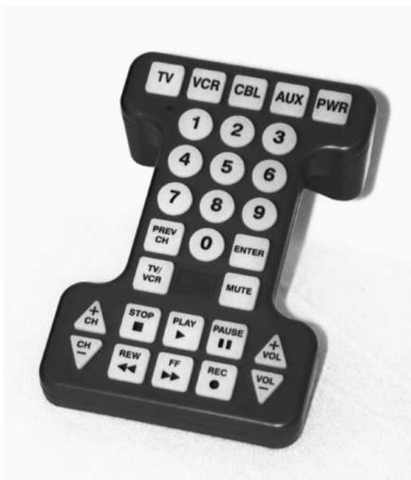
Figure 1. A remote control device with large buttons is easier to use for people who have arthritis or other difficulties with their hands.
