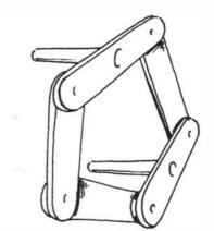
9-9. Closed kinematic chain of levers.
