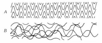
1—10. A – coherent, and B – incoherent light waves.
