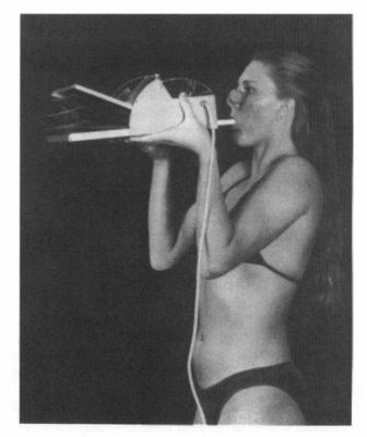
12—39. The Vitalor is an instrument to measure vital capacity and maximum expiratory flow rate.
