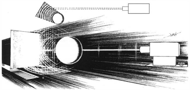
1—17. The image is reconstructed by the coherent light striking the hologram at the same reference beam creation angle. The image appears where the object originally was.
