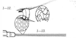
A flashlight and a laser are examples of incoherent and coherent light waves, respectively.
