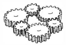
9-8. Closed kinematic chain of gears.
