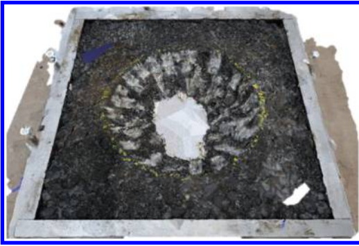
Figure 4. Laboratory manufactured pothole TIN at Stage 4, created and displayed in Zephyr.
