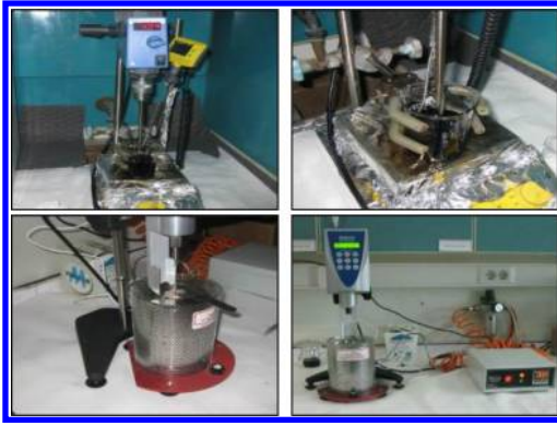
Figure 1. Viscosity measurement preparation and test setup.
