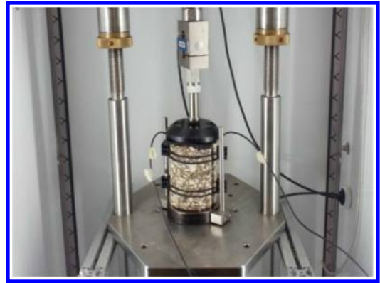
Figure 4. Cyclic compression test setup.
