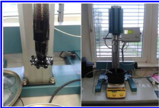
Figure 1. Cowles agitator (left) and mixer used (right) for the homogenisation of the bitumen ZycoTherm® mixture.
