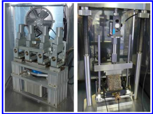
Figure 1a and 1b. Measuring device 4PB-PR and IT-CY test in Nottingham Asphalt Tester.
