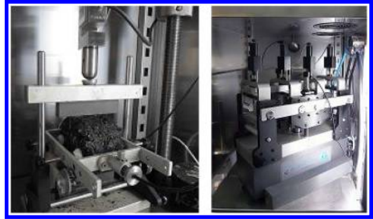
Figure 3. Stiffness (left) and fatigue test (right).
