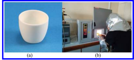
Figure 4. (a) High alumina crucible, (b) extraction of sample.
