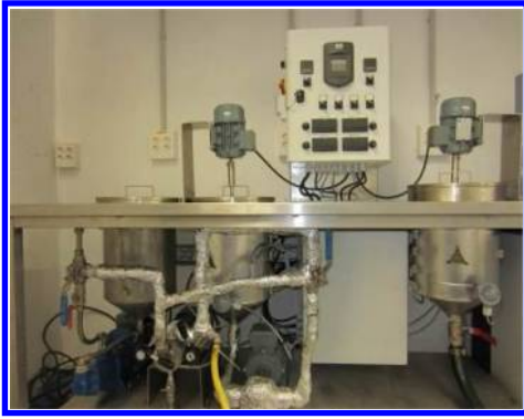
Figure 1. Asphalt binder modification laboratory plant.
