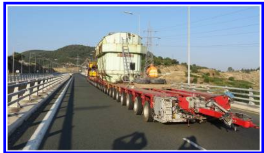
Figure 1. 24 axles overweight/oversize vehicle transporting energy generator over a bridge of Egnatia motorway.
