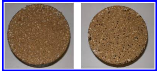
Figure 9. Very dense grade specimens: reference (left) and 1% capsules (right).
