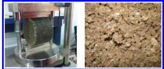
Figure 10. Core specimens after fracture by indirect tensile test.
