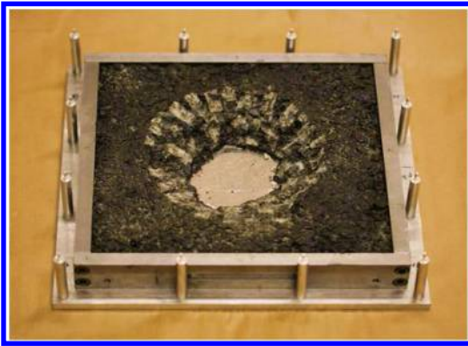
Figure 1. Calibrated steel framework of control points.
