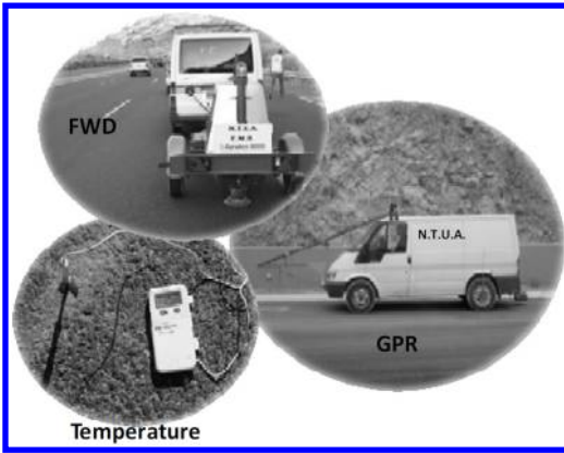
Figure 1. In situ road data collection.
