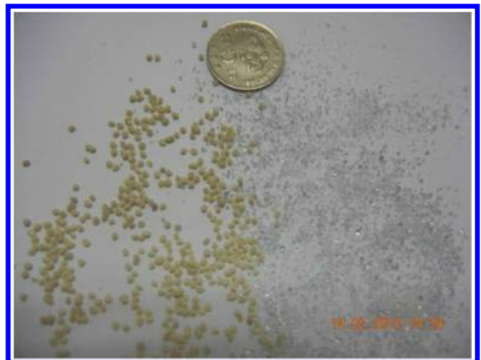
Figure 4. Comparison of size between glass beads and micro-crystalline ceramic beads.
