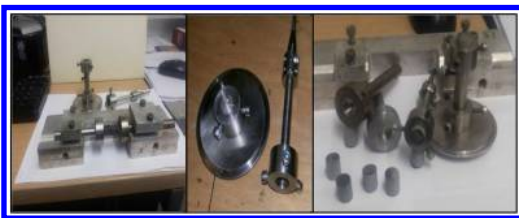
Figure 2. Aggregate steel holder and fixing device.
