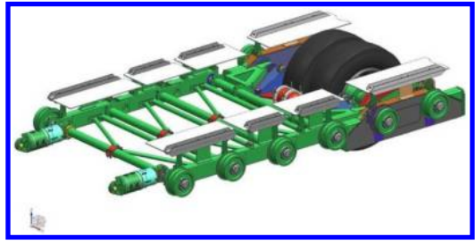
Figure 2. One of four Bogie inside the MLS10 (LMT Products (Pty) Ltd).
