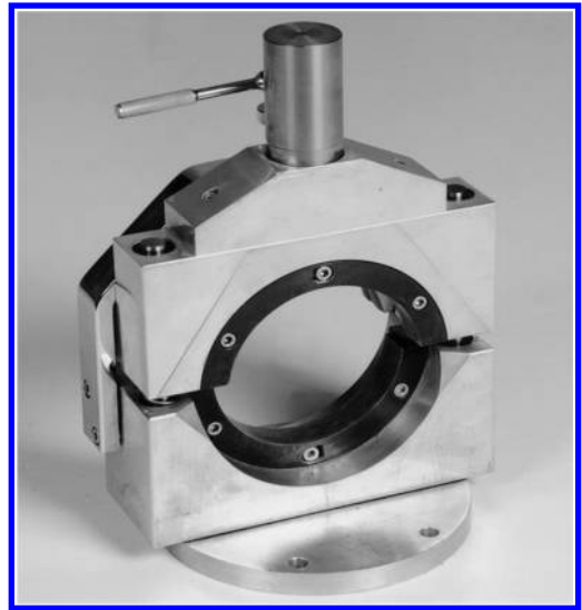
Figure 1. Shear bond test device according to Leutner (Leutner, 1978).
