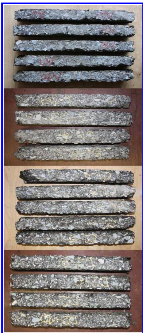
Figure 5. Damaged beam specimens (BCSM-BE, BCSM-FB, BSM-BE, BSM-FB) – before testing.
