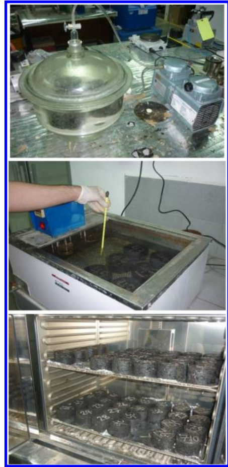
Figure 3. Moisture conditioning and long-term oven aging of samples.
