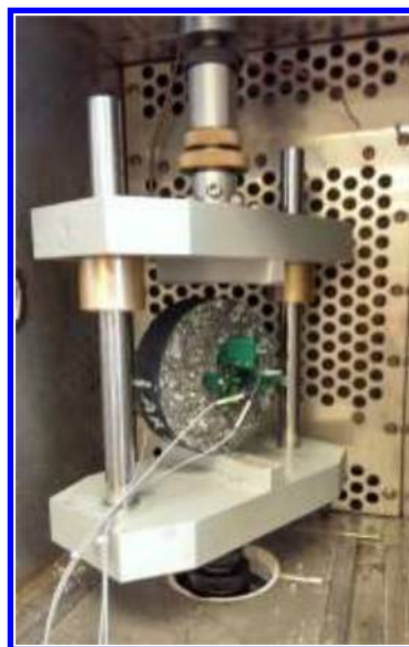
Figure 1. Indirect tensile test fixture, specimen and extensometers just prior to testing.
