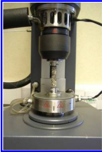
Figure 6. Small diameter core mounted on the rheometer.
