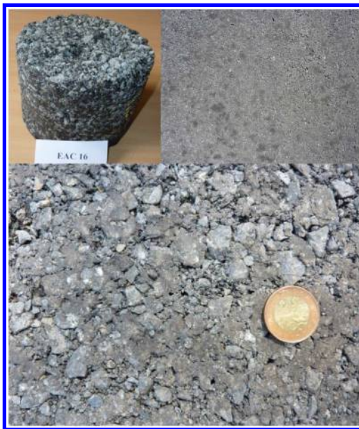
Figure 3. Examples of produced mix, including a test sample (mix from KMA 200) – example of aggregate coating quality.
