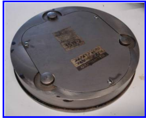
Figure 9. Gyratory load plate assembly.
