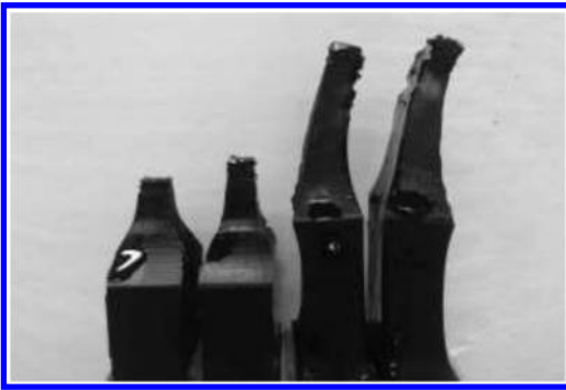
Figure 3. Images of polymer modified samples that failed through tearing.
