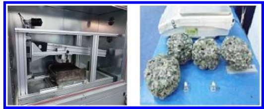
Figure 2. Wheel tracking test (left) and specimens after particle loss test.
