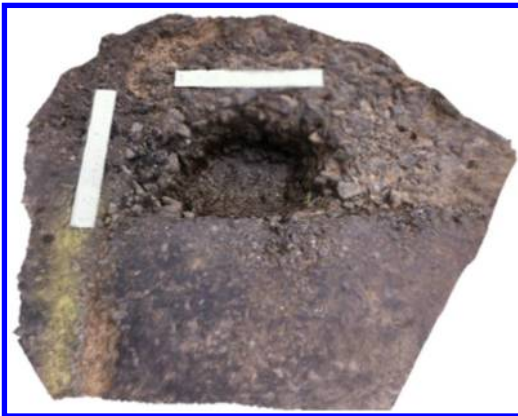
Figure 11. Real pothole TIN captured using Canon 6D camera device created and displayed in Zephyr.
