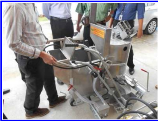
Figure 9. Applicator machine with double-drop facility.
