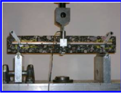
Figure 5. Flexural strength test set-up.
