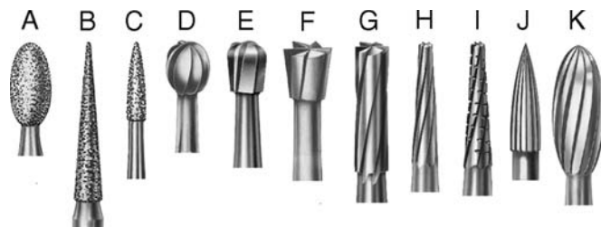
FIGURE 16.2 Names and shapes of dental burs. A. Egg or football diamond B. Needle diamond C. Flame diamond D. Round E. Pear F. Inverted cone G. Straight-fissure plain H. Tapered-fissure plain I. Tapered-fissure crosscut J. Needle finishing K. Egg or football finishing. (Courtesy of Brasseler USA)
