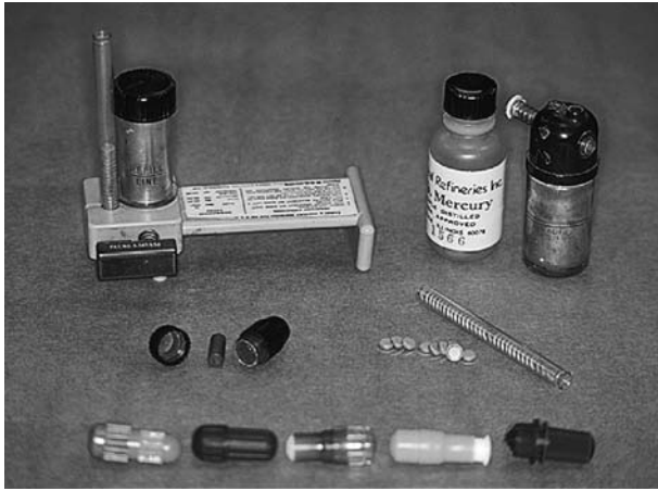
FIGURE 6.8 Several forms of amalgam alloy as supplied by their manufacturers. Top row (moving left to right). Alloy pellet and mercury dispenser, bulk mercury in a plastic bottle, mercury dispenser. Center row. Reusable capsule and amalgam alloy pellets. Bottom row. Several precapsulated amalgam products.
