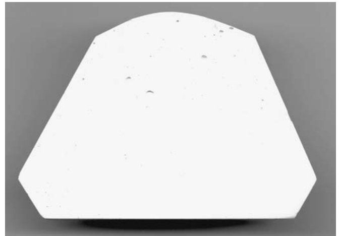
FIGURE 28.25 Pores and voids are present in the upper half of the base of this cast. In the lower half, the pores and voids have been filled and sanded for final finishing.
