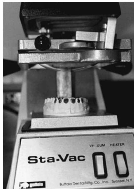
FIGURE 31.6 Stone model with facial reservoirs centered on the vacuum former. Warm resin is sagging below the frame.
