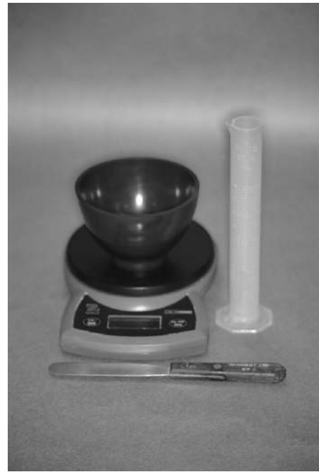
FIGURE 9.6 Equipment for mixing gypsum products: scale, rubber mixing bowl, graduated cylinder, and plaster spatula.
