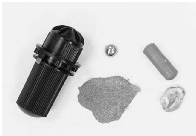
FIGURE 6.1 Starting at the left and moving clockwise: capsule, liquid mercury, pestle, freshly mixed amalgam, and powdered amalgam alloy.
