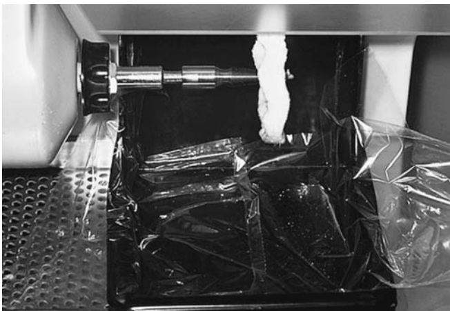
FIGURE 21.4 Dental lathe with sterile rag wheel attached and a single-use liner.
