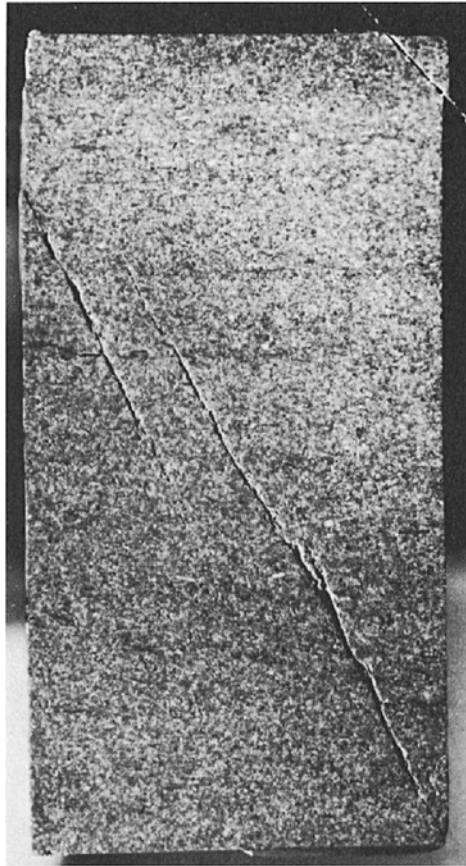
Figure 1.2.4 Macrofractures in a limestone under triaxial compression (courtesy of Dr. J.Labuz).
