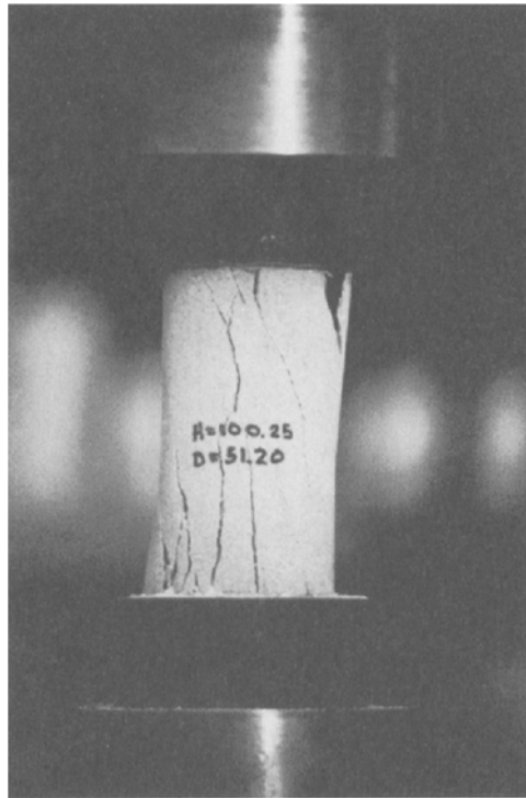
Figure 1.2.5 Failure by axial splitting of a Berea sandstone specimen loaded in uniaxial compression (courtesy of Dr. E.Papamichos).
