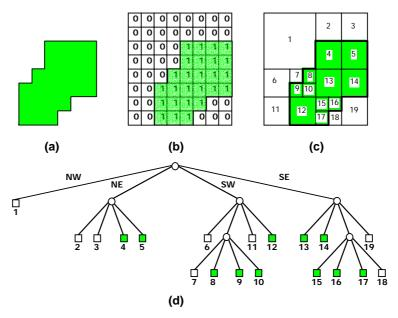
Figure 20: Sample (a) region, (b) its binary array, (c) its maximal blocks, and (d) the corresponding quadtree (after SAMET 1990a)
