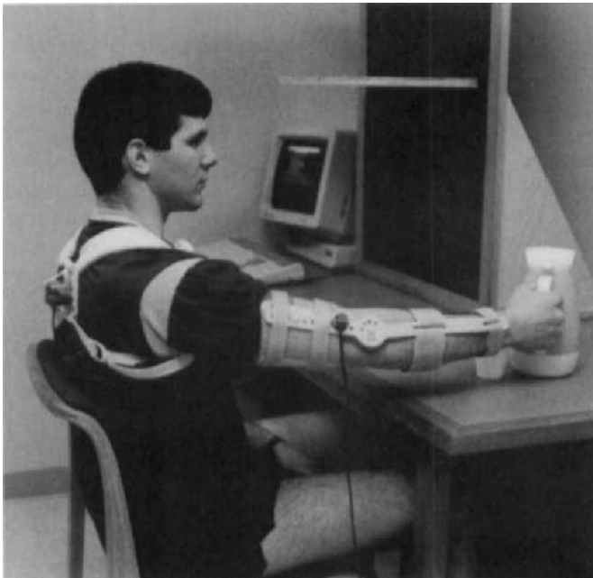
Figure 3. The electromagnetic tracking system. With source on the elbow brace and source attached on the thoracic spine, the motion of the shoulder complex was measured during reach activities. From [2]
