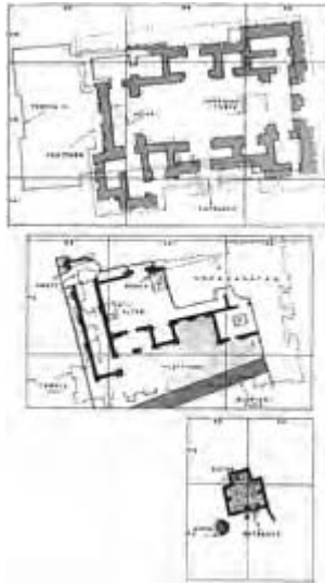
Figure 8.5 Temple plans characteristic of the three main phases recognized in the sounding at Eridu: top, 'Ubaid 4' (temple VII), middle, 'Ubaid 3' (temple IX) and, above, 'Ubaid 1' (temple XVI), dated respectively to c. 3800, 4100 and 4900 BC. Temple XVI (not shown) is no more than a chapel, but already has a niche for the altar and offering-table. (Lloyd 1978:42.)
