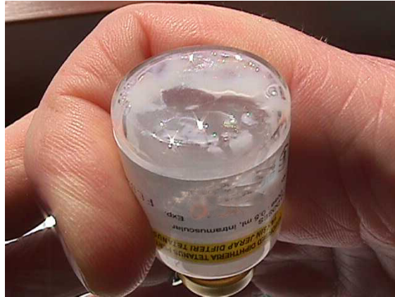
Fig. 10. Sub-zero temperature effect on DTP vaccine (after 10 minutes of vigorous shaking)
