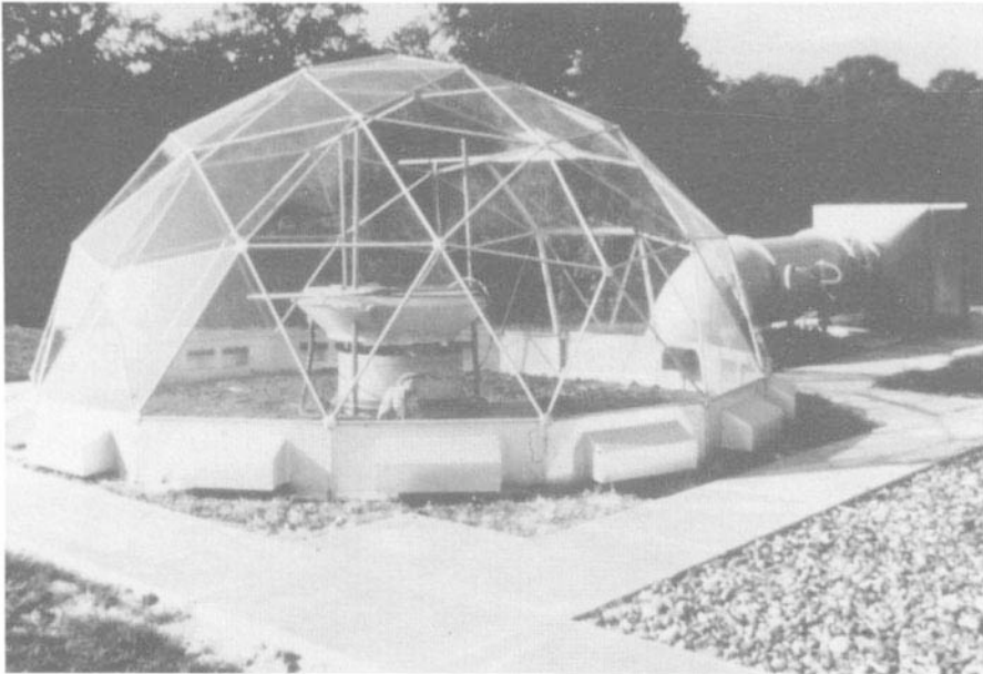
PLATE 2.2 A common way to examine how air pollutants affect plants is to grow them in Solardomes and expose them to different concentrations of pollutants. Alternatively one might take ambient air and filter it to see if current pollutant levels are having detrimental effects. Photograph: Andrew Farmer.
