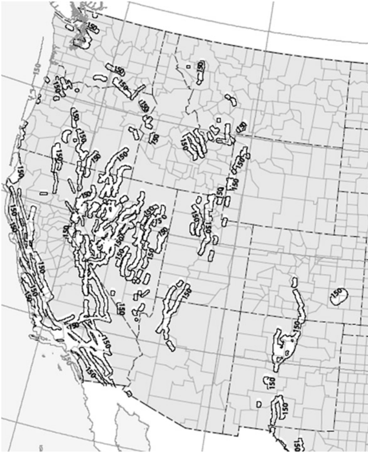
Fig. 4.8 Deterministic USGS contour map for short-period spectral acceleration ( T = 0.2 s) that is given separately in the 2009 NEHRP provisions and ASCE 7-10. Contours are in %g (modified from the 2009 edition of NEHRP provisions)
