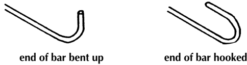
Figure 5.57 Ends of reinforcing rods.
