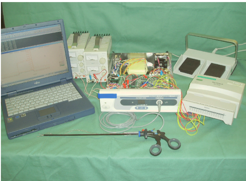
Fig. 13.1 The prototype hemostatic system used for the current experiments includes dissecting forceps for endoscopic operations, a power controller, a connecting cable, and a foot switch
