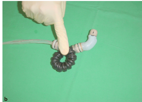
Fig. 11.10 The E 2 self-propelling endoscope is a pneumatically controlled inchworm that moves through the colon by a sequential adhering to the bowel wall and elongating/shortening the midsection. a Inchworm with imaging head and propelling body. b High flexibility
