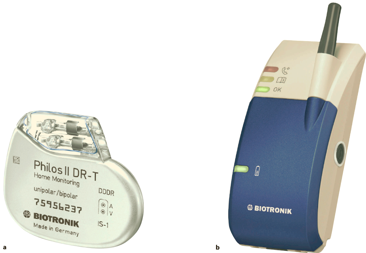
Fig. 11.1 Telemetric pacemaker for remote patient monitoring. Source: Biotronik GmbH, Berlin, Germany. a Pacemaker with telemetry units. b Mobile data transfer unit, like a cellular phone
