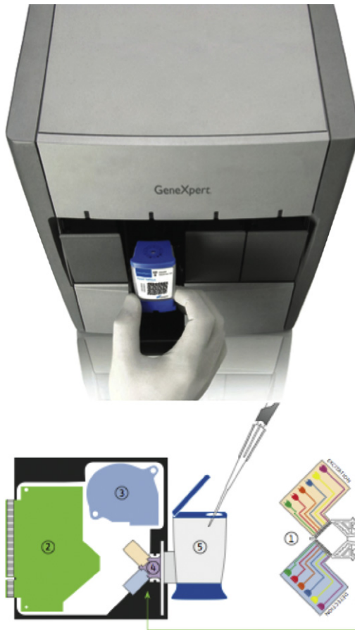
Fig. 3. The TB GeneXpert System (Cepheid) is a closed, self-contained, fully integrated, and automated nested real-time PCR platform for rapid diagnosis of TB and simultaneous confirmation of rifampicin resistance. The system is designed to purify, concentrate, detect, and identify targeted Mtb -specific nucleic acid sequences, thereby delivering answers directly from unprocessed samples. The sample is placed into a cartridge (5) and the targeted sequence is amplified by PCR (4); the optical PCR block detects and quantifies 6 different nucleic acid targets (1), and the circuitry (2) passes the information to a computer for display. The technology is suitable for use as a potential point-of-care test for use in microscopy centers and district hospitals. The key advantage, in contrast to the Hain assay, is a lower risk of contamination. (From Cepheid: www.cepheid.com ; with permission.)
