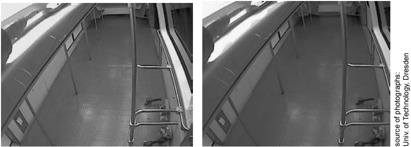
Figure 6: Detection example of the OEVD module (left: empty vehicle; right: person at the rear)
