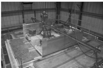
Figure 11: Floor Sample Over Furnace Photo: Bombardier/ Scott Moore, 2012
