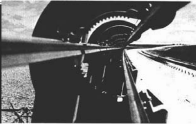
Image 12: 3-phase, al/ss v-contact power rails for TACV, Conductix Inc.
