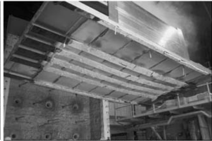
Figure 12: Underfloor After Test Photo: Bombardier/ Scott Moore, 2012
