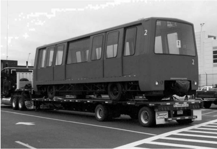
Figure 2-2: Installation of New Adtranz/Bombardier CX-100 Vehicles (photo courtesy of the Port of Seattle)
