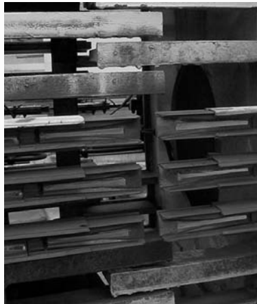
Image 24: Transfer caps are commonly used to manage collector shoes across switch gaps, Conductix, Inc.
