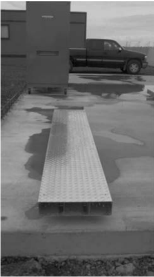
Figure 23: Cable Tray Mockup
