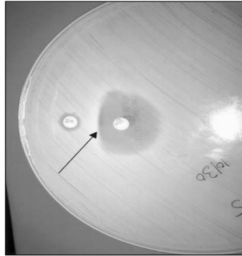
Figure 4. Double-disk diffusion “D” test to detect inducible clindamycin resistance in staphylococci based on induction of resistance by a 15 µg erythromycin disk placed 15-26 mm from a 2 µg clindamycin disk. Blunting of the inhibitory zone around the clindamycin disk forming a D shape denotes a positive test as indicated by the arrow. Isolates are reported as resistant to clindamycin irrespective of MICs determined prior to induction. Figure is reproduced by permission from reference 8.
