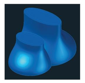
**FIGURE 17.26** Offsetting edges on the tops of the ventilation towers
