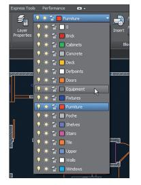
FIGURE 2.19 Making the Equipment layer current
