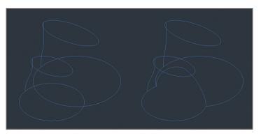
**FIGURE 17.22** Wireframe representations of two separate lofted ventilation towers (left) and a single object (right) created with Boolean union
