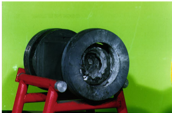
Fig. 12 Catching piston with projectile impact into steel plates
