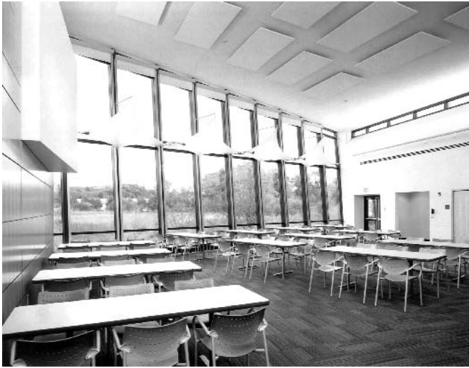
Figure 4-2 Example of north-facing assembly space that optimizes daylight harvesting while minimizing solar gain.
