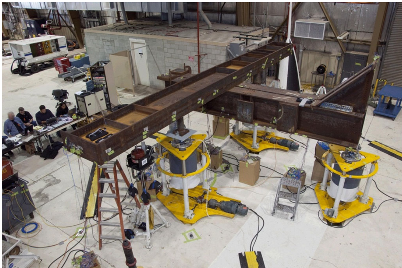
Fig. 10.2 The initial iron bird test article undergoing DIM testing
