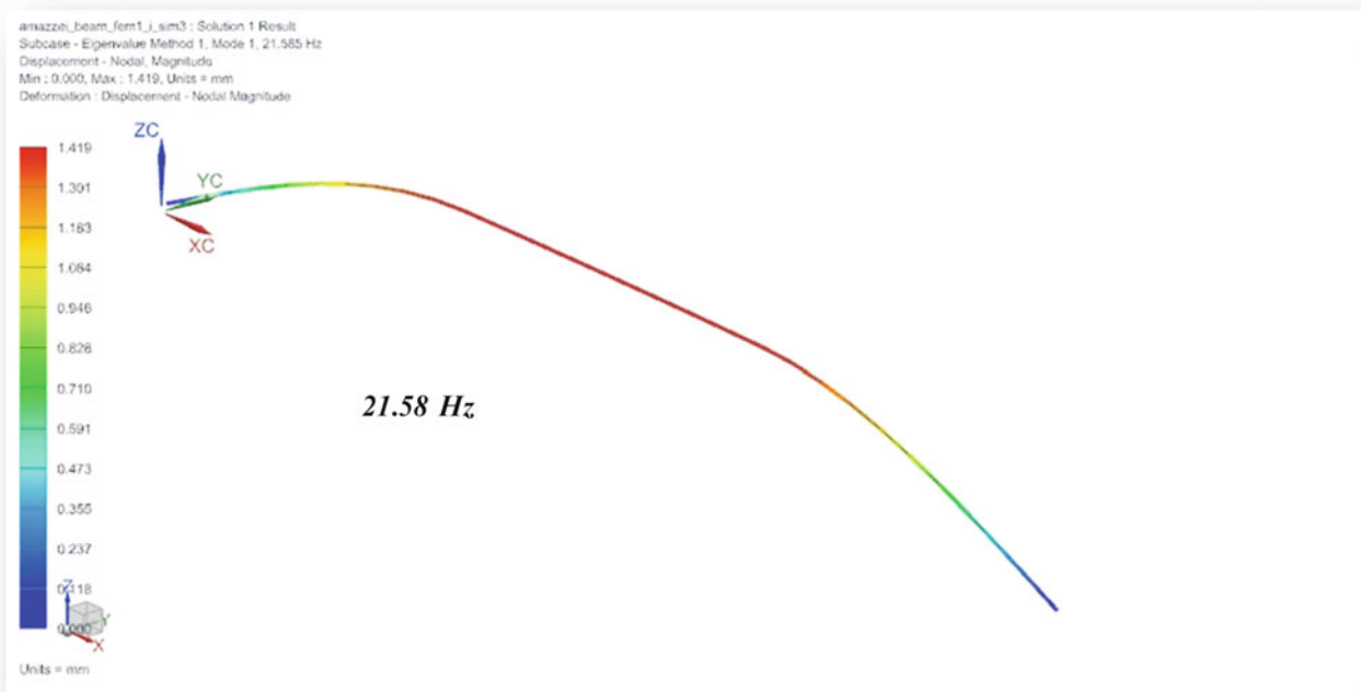
Fig. 20.15 First mode of pin-pin square non-uniform three-cell beam via FEM
