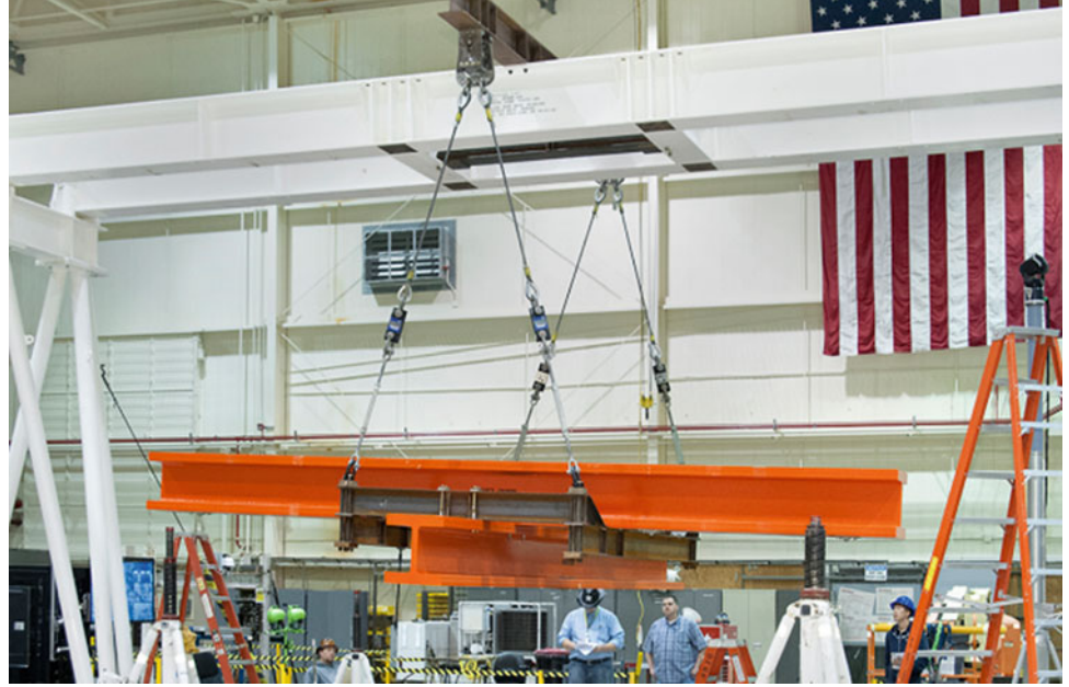
Fig. 10.5 The iron bird undergoing I_{xx} pendulum testing
