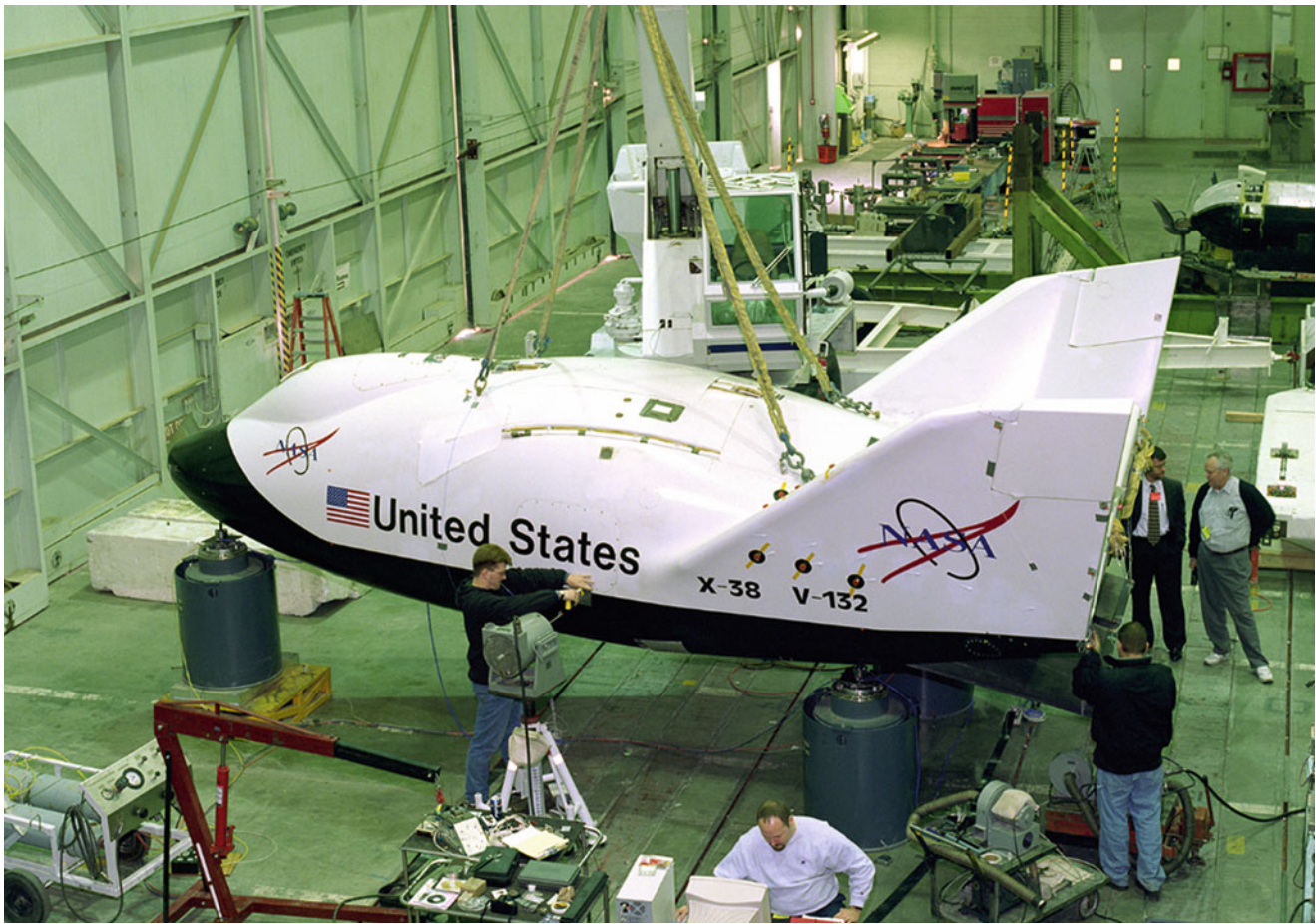
Fig. 10.1 The X-38 CRV undergoing DIM testing
