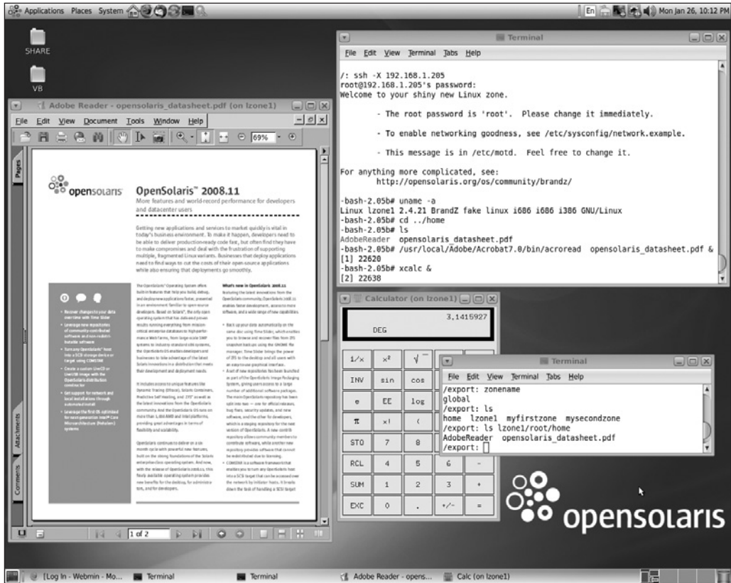
Figure 7-32. Running the Linux versions of acroread and xcalc in an lx -branded zone and displaying on the global zone desktop using X11 forwarding
