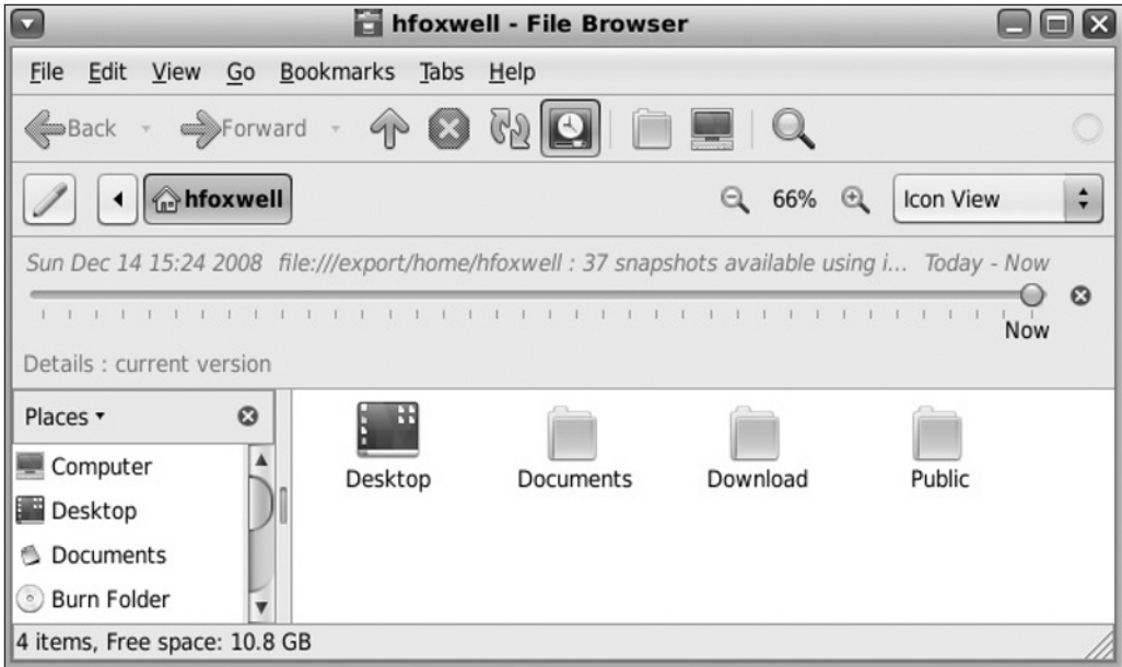
Figure 6-12. The Time Slider's slider bar, showing Time Slider's start time and date, the name of your file system, and the number of available snapshots
