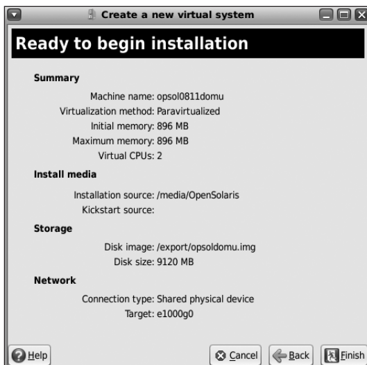
Figure 7-29. Ready to begin DomU VM installation
