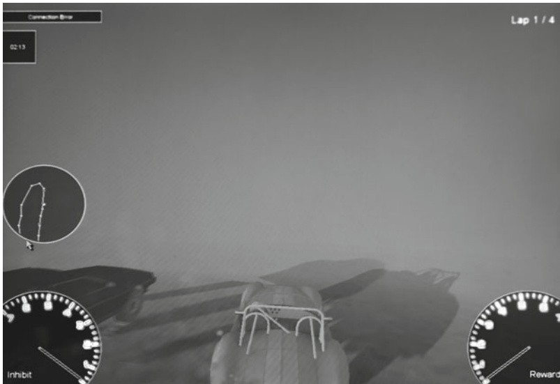
Fig. 2.1 Neurofeedback racing game. The client is connected to an EEG device that monitors the brainwave frequencies. If the ‘right’ frequencies are produced, the neurofeedback system makes the car speed up. If not, the car does not move, or is passed by another car (Used with permission of Roland Verment)
