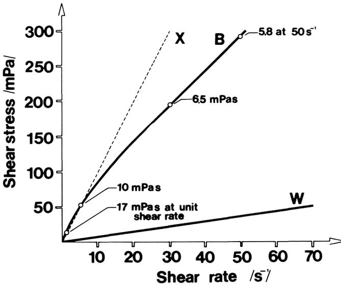
Figure 2.16. Flow curve for a normal blood at 37°C. Hematocrit = 0.40, plasma viscosity = 1.30 mPas. Straight lines are for Newtonian liquids, water (*W*) and an oil of 10 mPas viscosity (*X*).
