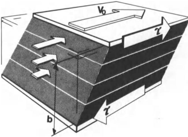
**Shear strain rate:**  $\dot{\gamma} = \frac{V_0}{b}$
