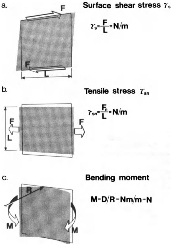
Figure 2.5. Definitions of the stresses  $\tau_s$ ,  $\tau_{sn}$  and the bending moment  $M$  in a membrane.  $D$  is a bending stiffness and  $R$  is a radius of curvature.
