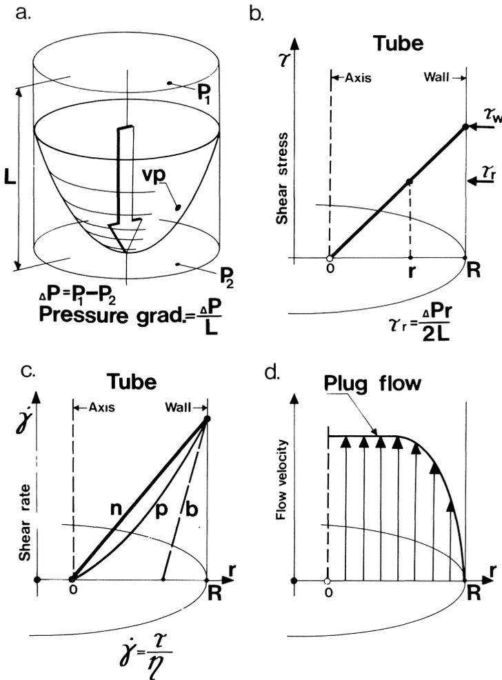
Figure 2.6. Tube flow. a: Pressure gradient in a tube is defined as  $\Delta p/L$ ; where  $\Delta p$  is the drop of pressure in a distance  $L$ . In a horizontal tube filled with Newtonian fluid there is no pressure-gradient without flow, and there can be no flow without pressure-gradient. The flow velocity in the tube varies as shown by the velocity profile ( $v_p$ ). The velocity is zero at the tube wall, and maximum at the tube axis.
