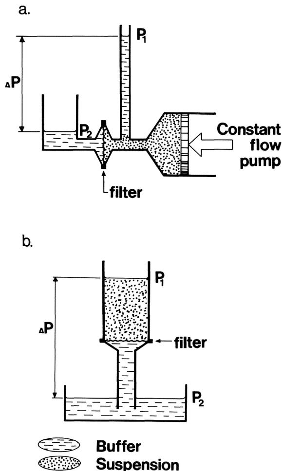
*Figure 2.13.* Filtration pressure. In a filtration system, pressure head is defined as the pressure difference between the upstream and downstream sides of the filter. Pressure loss in other parts of the system is supposed to be negligible. *a:* constant flow system; *b:* variable pressure head – variable flow system.  $p_1$  and  $p_2$  are upstream and downstream pressures, respectively.
