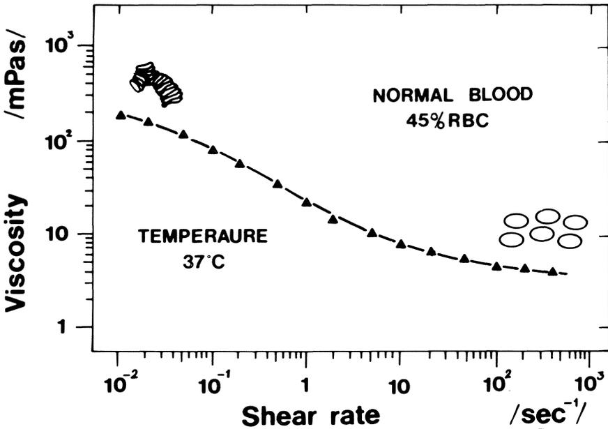
Figure 5.3. Logarithmic plot showing the relationship between the viscosity of normal human blood and shear rate. The insert sketches show the aggregation of red blood cells at low shear rates and their disaggregation and deformation at high shear rates. From (87).
