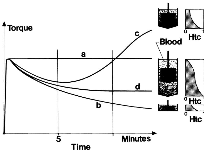
Figure 2.9. Aggregation and sedimentation in viscometry. Time-dependent changes in the blood sample placed in the viscometer result in artifactual changes of viscosity-readings at constant shear. Torque at constant rotational speed is plotted against time in three measuring systems. The small graphs on the right of each curve illustrate the assumed variation of red cell concentration (Htc) in the sheared zone of the sample.
