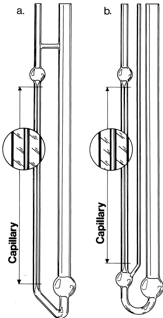
Figure 2.7. Simple glass tube viscometers.
