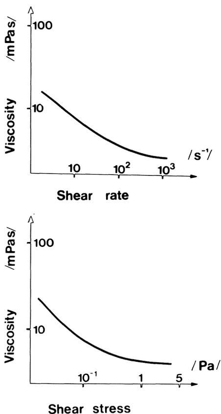
Figure 2.17. Viscosity of a normal blood sample. Anticoagulation with heparin, measuring temperature 37°C, hematocrit 0.44, and plasma viscosity 1.17 mPas.
