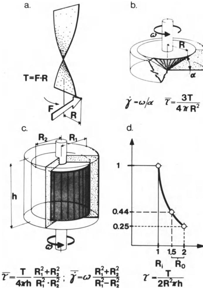
Figure 2.8. Rotational viscometry.  $\bar{\tau}$  and  $\bar{\dot{\gamma}}$  are the average shear stress and shear rate in the gap. The circular frequency  $\omega$  (radians/sec) is defined by  $\omega = 2\pi f$ , where  $f$  is the frequency of rotation (cycles/sec).
