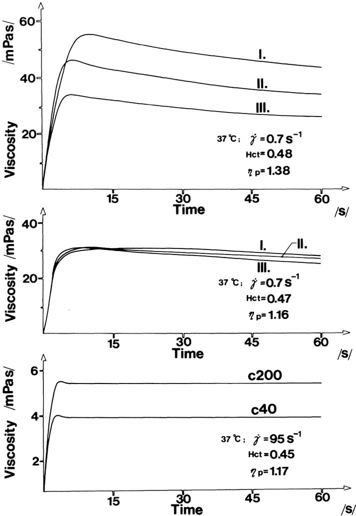
Figure 2.18. Whole blood viscosity at 37°C, plotted as function of time. Shear rate of  $0.7 \text{ s}^{-1}$  is applied in a Contraves LS-30 viscometer.
