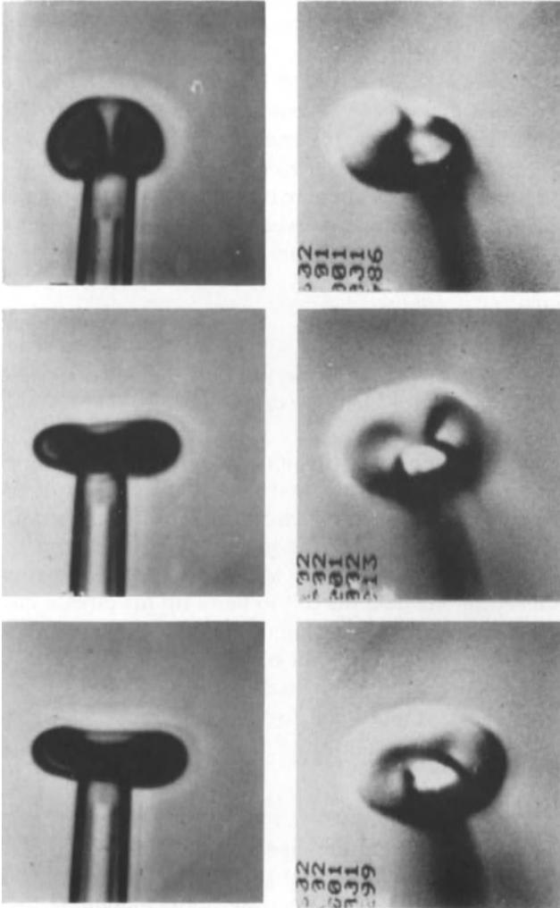
Figure 3.4 Illustrations of erythrocyte membrane extension followed by buckling. The pipette internal diameters are  $1 \mu\text{m}$ . The top panel shows the aspiration sequence as viewed from the side; the bottom panel shows a similar sequence viewed from above the cell with the use of a curved pipette. The figures to the right show the onset of buckling and folding of the cell.
