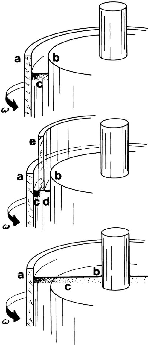
*Figure 2.10.* Surface film and guard ring. A viscous (or viscoelastic) surface film of adsorbed proteins builds up at the air-blood (and also at an oil-blood) interface. *a*: rotating-part of the measuring head; *b*: sensor-part of the measuring head; *c*: sheared surface-film; *d*: unsheared surface-film; *e*: guard ring.
