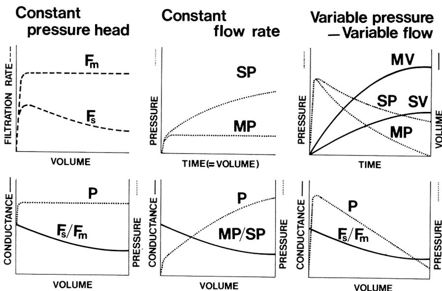
Figure 2.15. Analysis of filtration curves. The quantifying of filter blockage is required for the assessment of red cell deformability in filtration systems. This can be achieved in most blood filtration tests, as shown for all three types of blood filtration methods.
