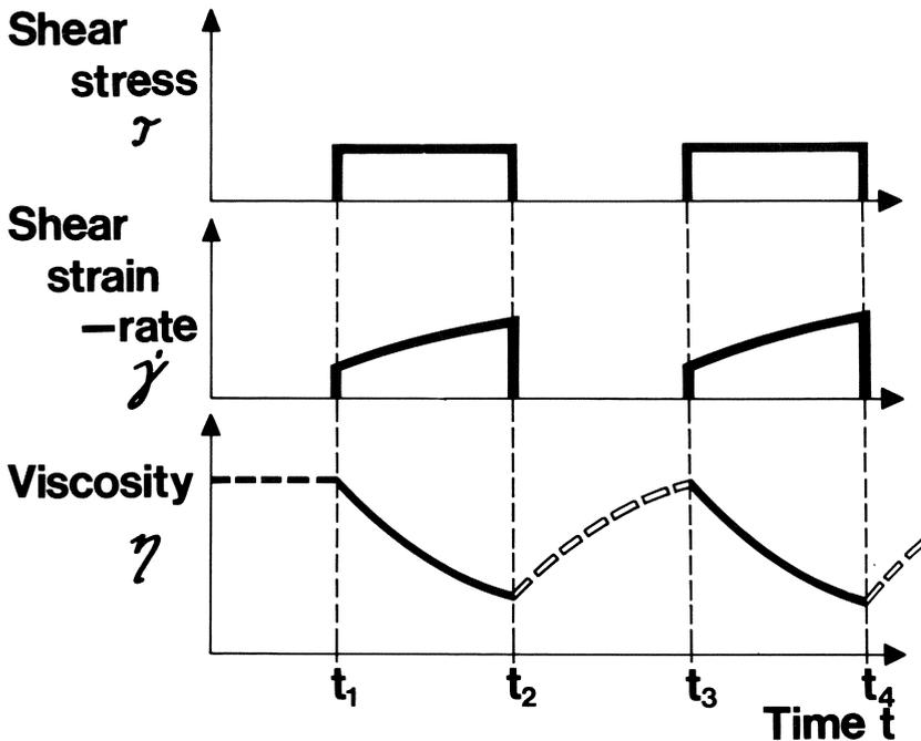
*Figure 2.4.* Response of a thixotropic fluid to intermittent shear stress. When a step change in shear stress is applied, the shearing of the sample results in progressive degradation of the internal structure of the fluid and the viscosity decreases in time. When the shear stress is removed the internal structure reverts to its original form. The dotted portions of the viscosity curves show the initial viscosity that would be observed if a shear stress were suddenly applied.
