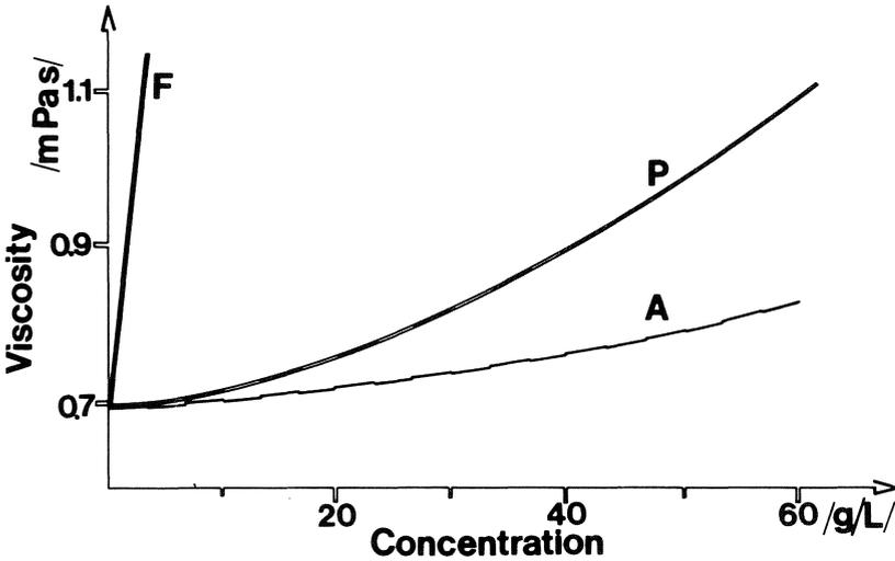
Figure 2.19. Viscosity of protein solutions plotted against concentration as measured at 37°C in a Harkness viscometer. *A*: with albumin in buffer; *P*: plasma diluted with buffer; *F*: with fibrinogen in buffer.
