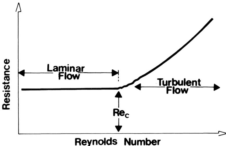
Figure 5.2. Effects of Reynolds number on flow resistance. Note the increase in resistance when the flow pattern undergoes transition from laminar to turbulent at the critical Reynolds number ( $Re_c$ ). As discussed in the text,  $Re_c$  is a function of the geometry of the flow system.
