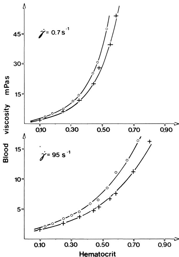
Figure 2.22. Hematocrit – viscosity relationships. + : a healthy subject, plasma viscosity 1.16 mPas; o: heart-infarction patient, plasma viscosity 1.53 mPas. Reconstituted samples measured at shear rates  $0.7 \text{ s}^{-1}$  (upper plot) and  $95 \text{ s}^{-1}$  (lower plot). Measurements were carried out in a Contraves LS-30 at  $37^\circ\text{C}$ . Semilogarithmic regression curves were fitted to each set of samples as shown by the curves.
