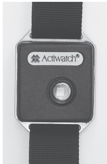
FIGURE 2.48 Wristwatch photo-sensitive data logger. Wristwatch data loggers are convenient instruments for monitoring locomotor activity in human subjects. Units with photocells also allow the monitoring of light-exposure patterns. (Source: Image courtesy of the Mini-Mitter Company, Bend, OR.)
