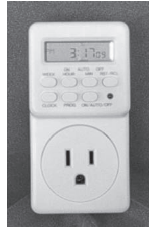
FIGURE 2.51 Controlling the light–dark cycle. An electronic timer such as this one provides a simple way to turn lights on and off at desired times in a laboratory setting.
