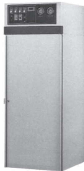
FIGURE 2.52 Controlling ambient temperature. Environmental chambers (ventilated heated incubators) such as this one provide a reliable way to control ambient temperature in a laboratory setting. Some models have programmable timers that allow the generation of daily cycles of ambient temperature.
