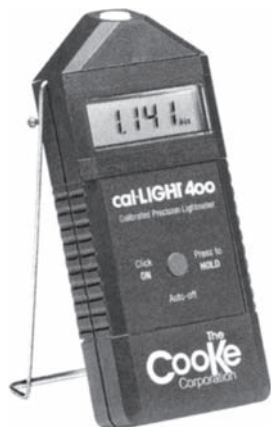
FIGURE 2.47 A photometer. Photometers are instruments used to measure illuminance (light intensity in lux). (Source: Image courtesy of the Cooke Corporation, Auburn Hills, MI.)
