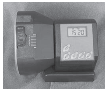
FIGURE 2.53 Controlling food availability. Automated fish feeders such as this one provide a simple way to control feeding time for small animals in a laboratory setting.
