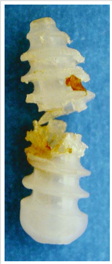
Figure 7.19. Broken femoral interference screw. (Reprinted from Sanchis-Alfonso, V, and M Tintó-Pedrerol, Femoral interference screw divergence after anterior cruciate ligament reconstruction provoking severe anterior knee pain, Arthroscopy 2004; 20: 528–531, with permission from Arthroscopy Association of North America.)
