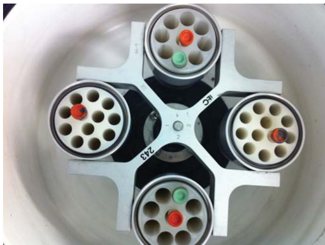
Figure 4.4 The centrifuge should be balanced with similar tubes filled with a similar volume of liquid to match the volume of blood.
