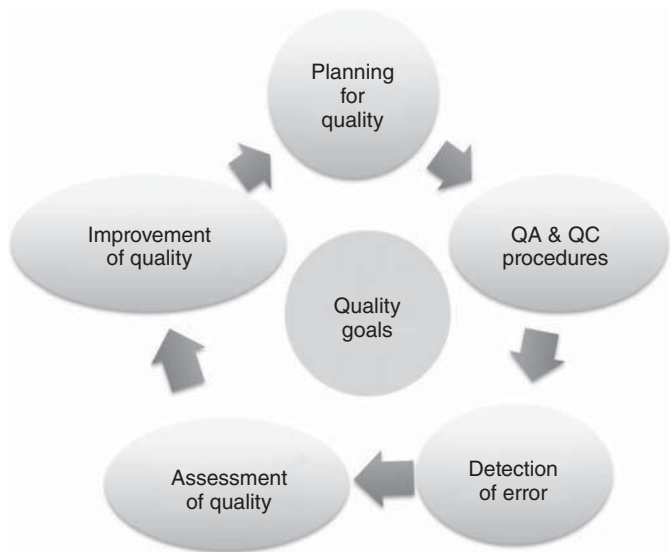
Figure 7.2 The lynchpin of the quality cycle is having specific quality goals that allow planning for quality. From there, QA/QC procedures can be implemented, monitored, and assessed, with improvements made as needed on a continual basis. When error is detected, efficacy of corrective actions should be assessed and documented.
