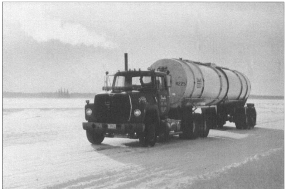
Figure 12.2.2 Heavy Truck on Ice Road. This truck and its load of diesel fuel weigh approximately 36,000 kg. It is on the ice road atop Island Lake headed north to the community of Garden Hill. (Photograph: R.H. Foster)
