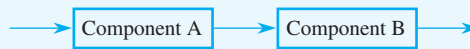
Figure 5.9 A two-component series system, which functions correctly only if both components function correctly
