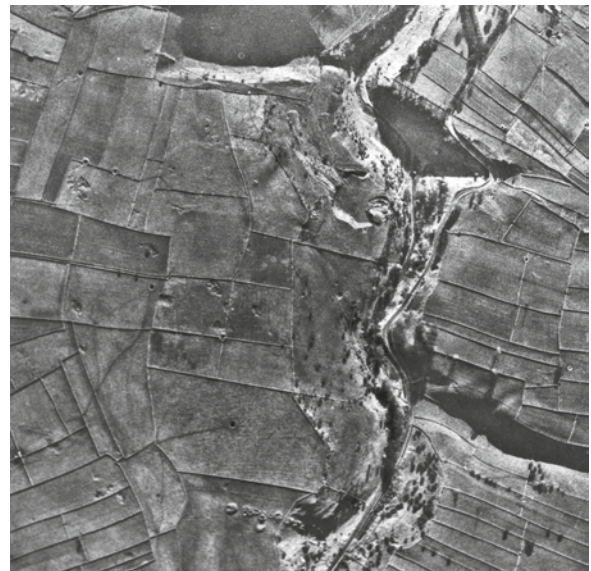
Fig. 3.1 Internal drainage in limestone. (Aerial photograph courtesy of Aerofilms Ltd.)
