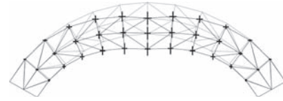
Figure 4. Range variability of nodal displacements, represented by tick segments, when all the elements have the elastic modulus defined by an interval variables with radius \Delta E = 0.3E_0 .
