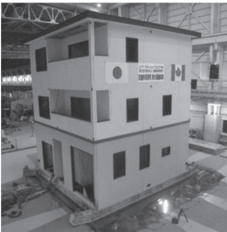
Figure 1. A three-story post-and-beam timber building and the PB3D model.
