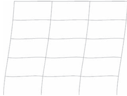
Figure 1. Office building MRF: Fundamental period = 1.27 s.
