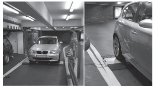
Figure 2. Load measurements at the Hauptwache multi-storey car park in Frankfurt am main.
