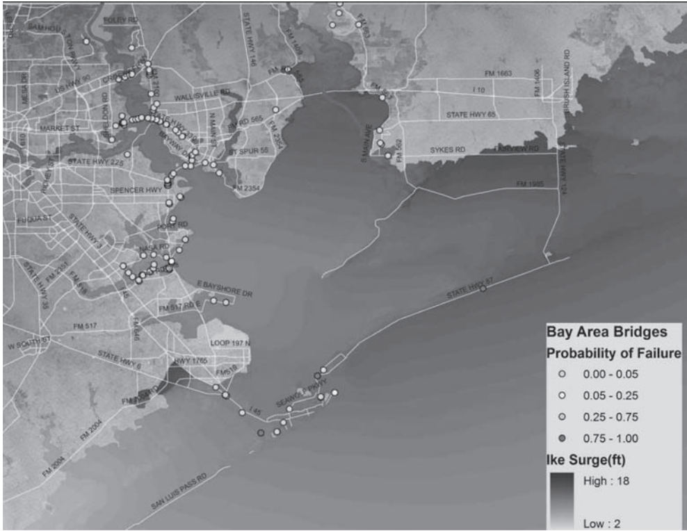
Figure 2. Probability of failure of bridges in Houston/Galveston for the Hurricane Ike scenario.
