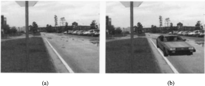
Figure 1 a) live scene, b) the result of inserting a virtual vehicle into the live scenes.
