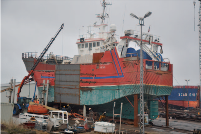
Fig. 2.4 The new regulation allowed operators to invest in fishing rights and to reorganize their operations and vessels to fit the new amount of quota. The photo shows a vessel being rebuilt and enlarged after having accumulated quota from other vessels. Photo: (Jeppe Høst)
