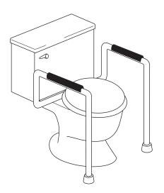
*Grab or safety bar*: steel bars of varying lengths can be placed in the tub and shower to assist with getting in and out of the shower or tub. Figure 10.15 shows grab bars, which are often found in the bathroom and next to a toilet to assist with moving on and off the toilet. Bars should be sturdy enough to hold the weight of the person using them; they provide support and help the care recipient maintain balance.
