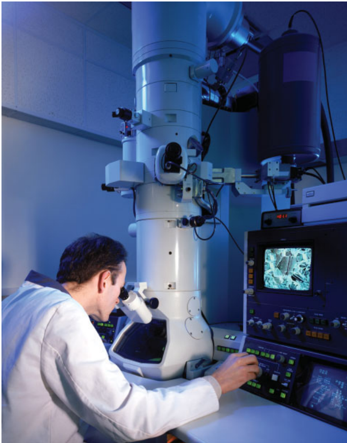
FIGURE 3.4 A transmission electron microscope.
