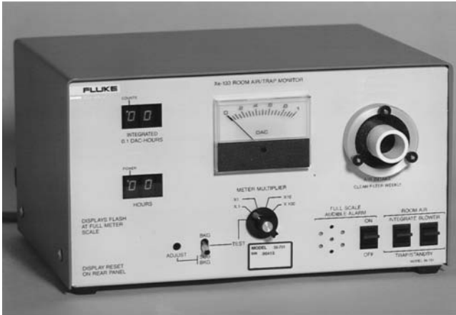
FIGURE 7.2 Alarm GM monitor specially designed for continuous air monitoring in the pulmonary ventilation room. (Courtesy of Fluke Biomedical, Cleveland, OH.)
