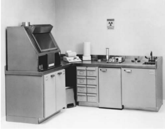
FIGURE 5.2 A view of the radiopharmacy or hot lab. A glove box appears on the left, a dose calibrator on the center, and a lavatory on the right. There are shielded cabinets and shielded drawers under the counters. (Courtesy of Fluke Biomedical, Cleveland, OH.)
