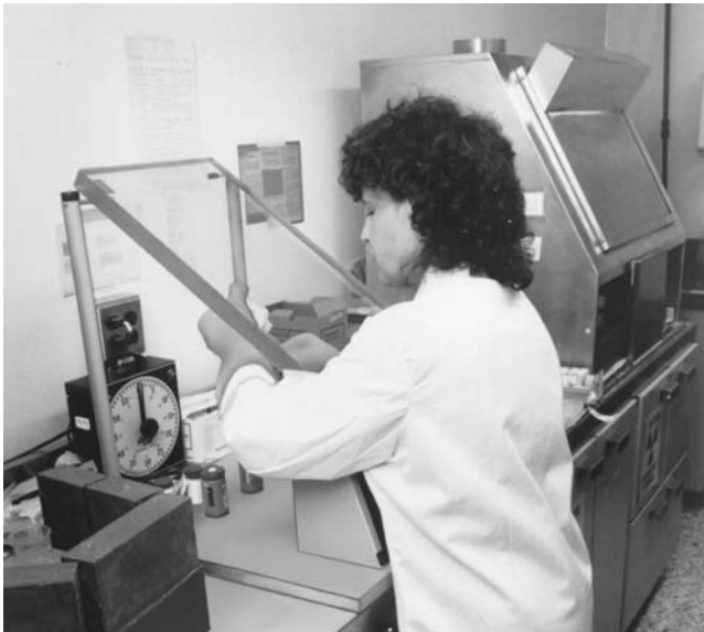
FIGURE 5.3 Behind a lead-glass shield, a radiopharmacist draws a dosage of a radiopharmaceutical for a patient. (Courtesy of Fluke Biomedical, Cleveland, OH.)
