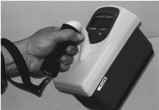
FIGURE 7.3 A state-of-the-art ionization chamber survey meter for monitoring of alpha, beta, gamma, and x-ray radiation. (Courtesy of Fluke Biomedical, Cleveland, OH.)
