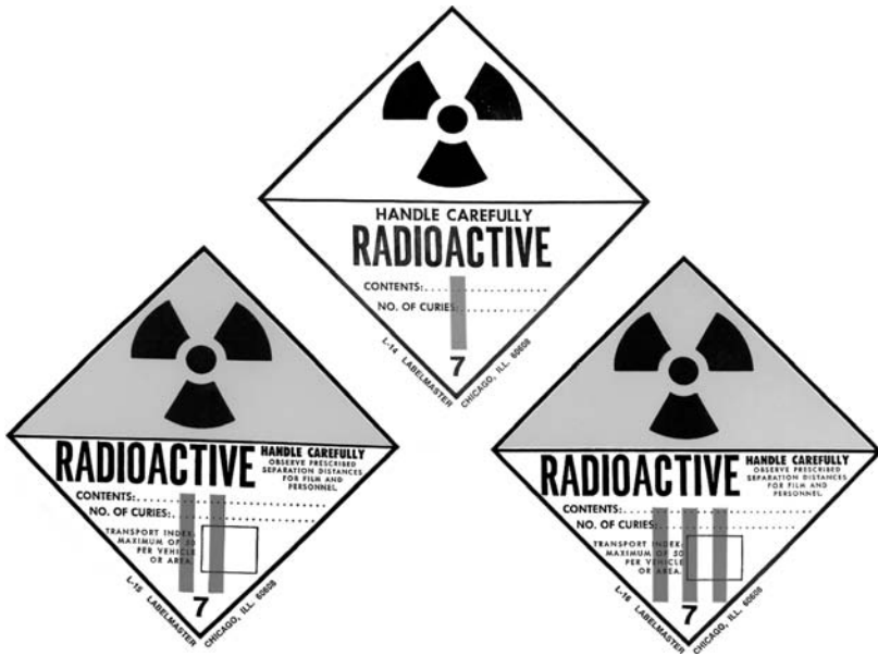
FIGURE 3.2 Labels authorized by the Department of Transportation for packages containing medical radiopharmaceuticals. For categories II and III, the top of each label has a yellow background.
