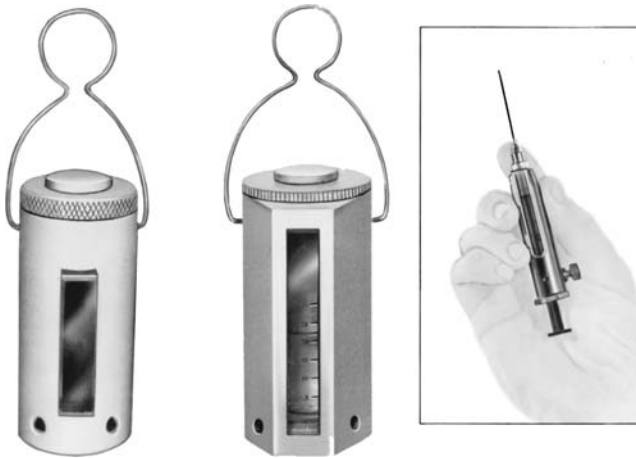
FIGURE 5.5 Two lead shielding devices for multidosage vials (left) and a tungsten shield for hypodermic syringes (right). All items shown have lead-glass windows. (Courtesy of Fluke Biomedical, Cleveland, OH.)
