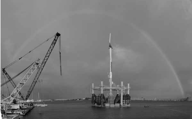
16.31 Large-scale prototype tension leg platform (© Blue H Technologies BV).
