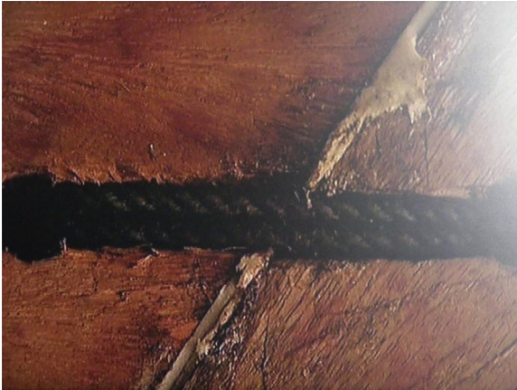
Figure 15.2 The traditional method of making sailboats from trees grown on the Islands of Micronesia is by gluing and stitching planks with natural fibre.
