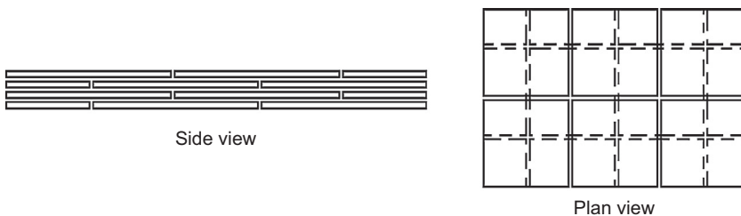
Figure 28.16 Possible arrangements for spreading joints throughout recycled material.
