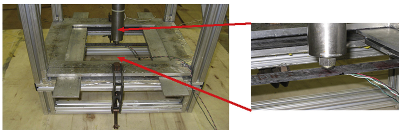
Figure 24.42 Test sample placed on impact test machine.
