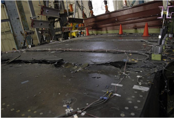
Figure 15.3 Full-scale break test of the Boeing's 787 Dreamliner Wing. The structural flaw in was found ca. May 2009. Stresses at the ends of the long rods that stiffen the upper wing skin panels caused the fibrous layers of the composite to delaminate. Inside the fuselage, on the other side of where each wing joins the body of the aircraft, is the centre wing box constructed much like the outer wing, with composite skin panels stiffened by composite stringers. The upper and lower surfaces and wing spars are made from the same composite material as the fuselage, while the wing ribs are machined from single pieces of aluminium.
