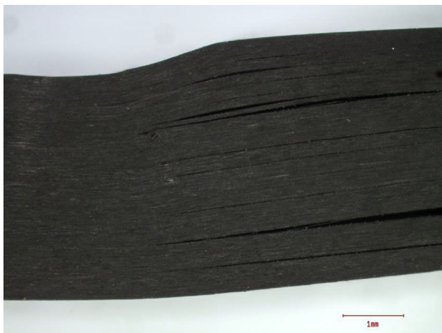
Figure 21.5 Delamination in an epoxy carbon short beam shear test.
