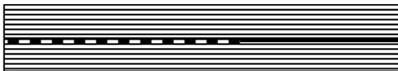
Figure 24.32 Side view of the tested sample with carbon nanotubes (CNT) introduced at the interface.
