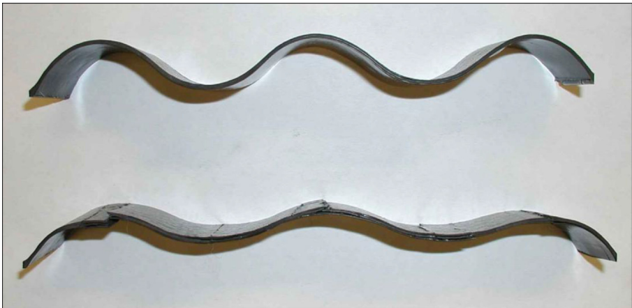
Figure 28.14 SE-84 LV corrugated plate (top) before recycling and (bottom) after forming at high temperature (F + H).
