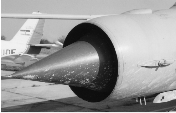
Figure 23.1 Impact-induced mechanical damage of inlet cone of a MiG-21bis fighter aircraft. Courtesy Moma Stanojlovic Company.
