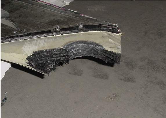
Figure 15.4 An American Airlines Airbus A300-600 had its vertical carbon fibre fin blown away during the take-off stage, with disastrous consequences.
