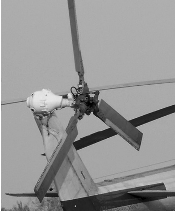
Figure 23.5 Heavy transport multipurpose helicopter: the tail rotor blades. Courtesy Moma Stanojlovic Company.
