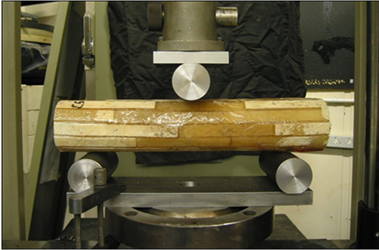
Figure 28.23 Three-point bending of the tubes.
