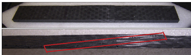
Figure 24.23 Specimen constructed with scarf joint.
