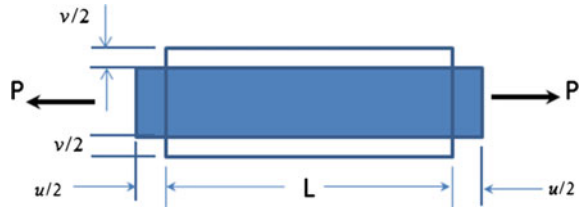
Fig. 6.1 Tensile loading of a bar
