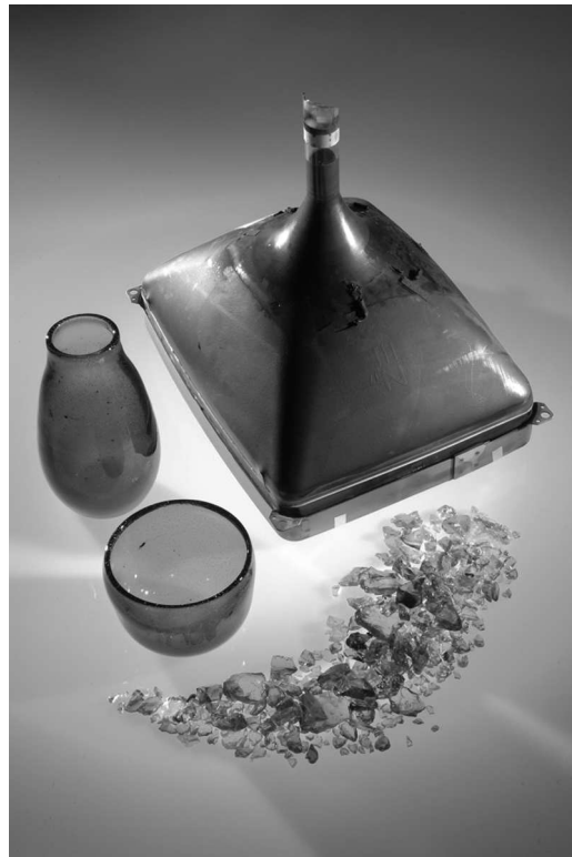
Figure 6 An end-of-life cathode ray tube, granulated CRT glass and a product made from this glass after the lead has been removed. (Courtesy NuLife Glass Ltd.)
