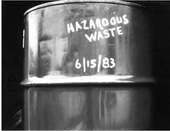
FIGURE 5.5 Dating accumulation container, satellite accumulation point, or temporary storage area. (From the Arizona Department of Environmental Quality.)
