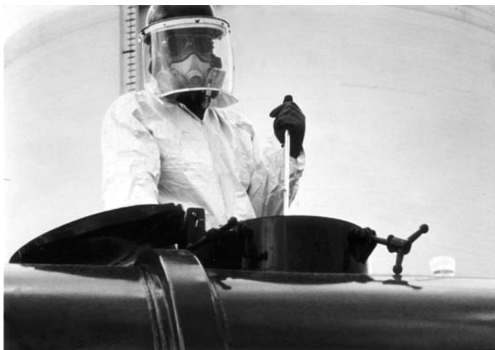
FIGURE 10.8 Sampling liquid waste with standard laboratory glass tubing. (Courtesy of Safety-Kleen Corporation.)
