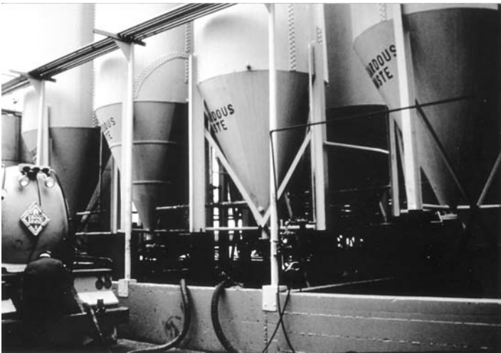
FIGURE 7.9 Gravity separation cones. (From ROMIC Chemical Corporation, 2081 Bay Road, Palo Alto, CA 94303. With permission.)
