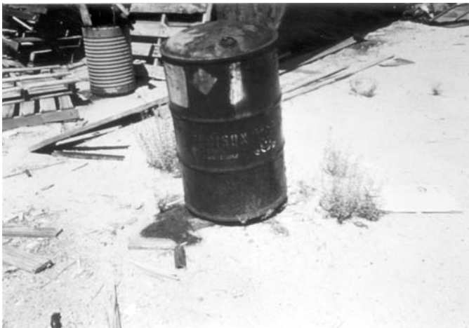
FIGURE 10.2 Bulged drum. (From the Arizona Department of Environmental Quality.)
