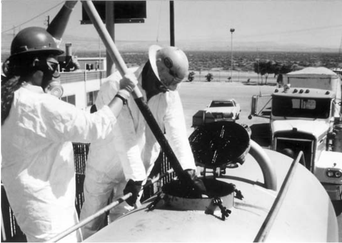
FIGURE 10.6 Single-use “Colawassa” sampler in use. (Courtesy of Safety-Kleen Corporation.)
