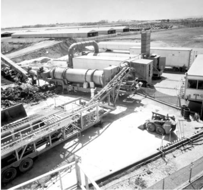
FIGURE 11.17 Transportable low-temperature thermal desorption unit. (From URS Corporation, 100 California Street, San Francisco, CA 94111-4529. With permission.)
