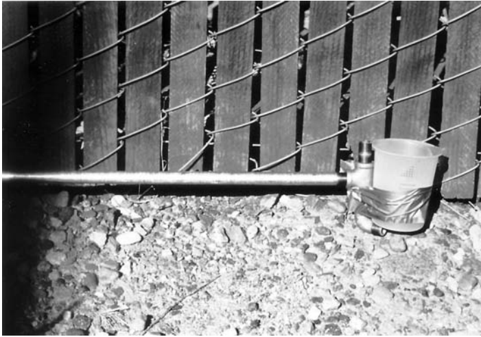
FIGURE 10.10 Makeshift dipper using improper materials. (From the Arizona Department of Environmental Quality.)
