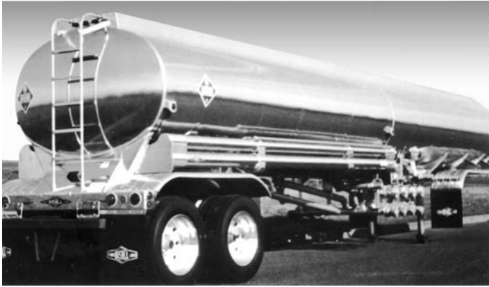
FIGURE 6.1 DOT specification MC-306 tank trailer for transporting combustible and flammable materials.
