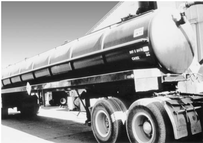
FIGURE 6.2 DOT specification MC-310 tank trailer for transporting corrosive materials.
