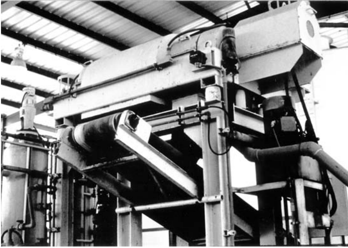
FIGURE 7.8 Centrifuge. Component of a hazardous waste solidification system.
