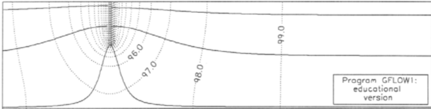
Figure 4.7: Piezometric contours and streamlines in a cross-section over a partially penetrating well in a confined aquifer. (GFLOW1 data file proble41.dat )
