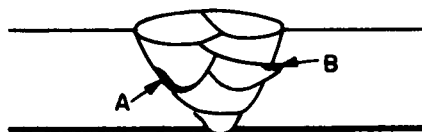
FIG. 15.2. Slag inclusions, between passes at A and at undercut at B.
